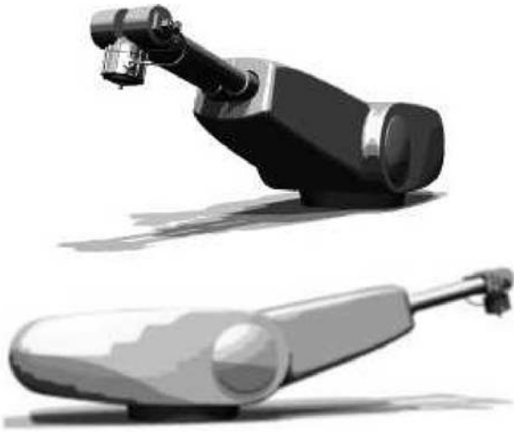
Figure 5.13 The Unimate Robot, introduced in 1961 (reproduced from computer animation).
