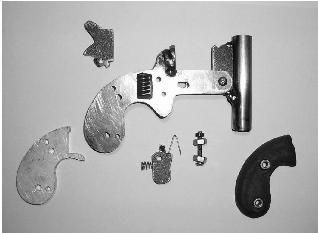
Disassembled: note the rudimentary barrel release latch consisting of a bolt and three nuts.
