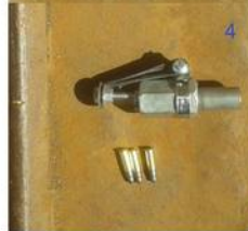
Pic5: The striker assembly. A piece of bicycle tire makes for an excellent spring. One washer has a notch to help the rubber band orient itself. Note that the band has ruptured after heavy use (100 shots), replacing it takes less than half a minute.
