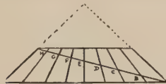
FIG. 79.—The width of eight squares lying flat marked off by receding lines and intersected by a diagonal.
