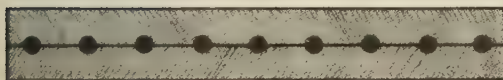
A second grooved and glued slat is placed on top, forming a sandwich, and held under pressure until the glue dries.
