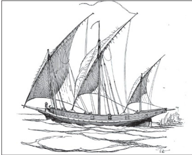
Figure 3.3. The lateen rig. Source: Pearson Scott Foresman archive, released to public domain.
