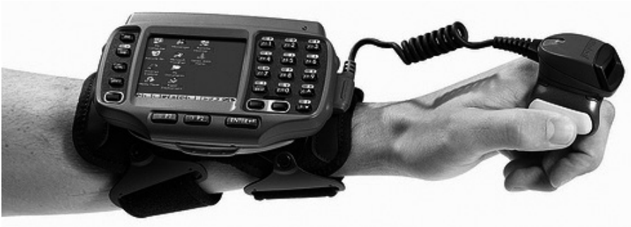
Picking scanner that told you what to pick as well as measuring your speed
