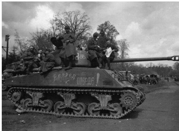
An M4A2 (76mm) in 1945 in Eastern Europe. The Soviets disliked the early gasoline-engine Shermans received from the Western Allies in the earlier years of the war and requested M4A2 models with diesel engines. A total of 4,252 M4A2s were received from the US, evenly split between 75mm and 76mm versions. (US Army)
