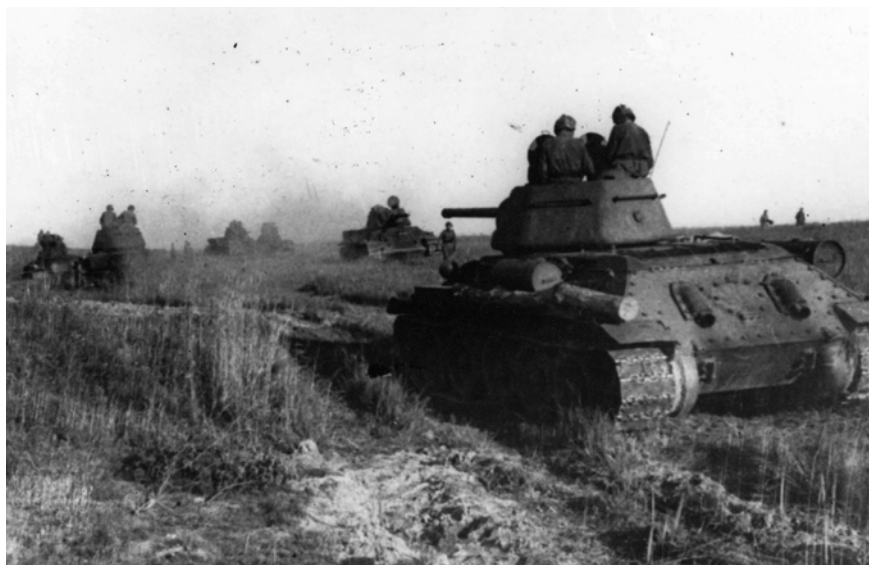
76mm-armed T-34s moving through the arid terrain faced by many Soviet formations during the campaign. The 6th Guards Tank Army found that the weight of several tanks driving close together could break through the top crust and bog down in the softer sand beneath, leading the units to spread out for the advance. (From the fonds of the RGAKFD in Krasnogorsk via Stavka)
