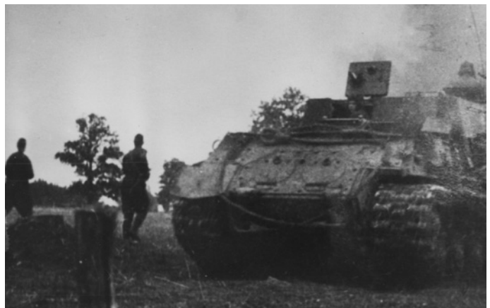
A rear view of an ISU-152 SPG on the advance with infantry support. Unlike almost all Soviet AFVs, the ISU-152 had a relatively roomy crew compartment and a variety of access hatches. Here, the loader looks out from his large, two-piece hatch while the vehicle commander surveys the way forward. (Courtesy of the Central Museum of the Armed Forces, Moscow, via Stavka)
