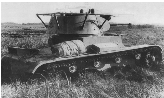
A late-model T-26 with sloped turret armor and the clothesline radio antenna. Some T-26s were produced in 1940 with more modern whip antennas. This T-26 does not have the rear-firing machine gun mounted in some versions to defend against infantry attack from the rear. (From the fonds of the RGAKFD in Krasnogorsk via Stavka)
