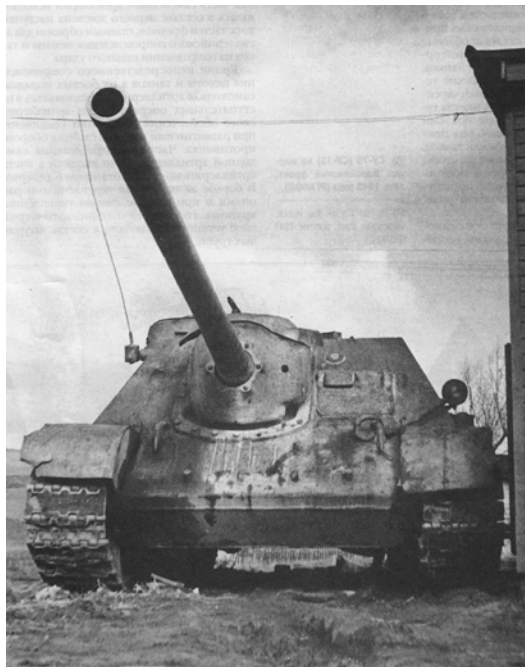
A head-on view of an SU-100. Like the other Soviet SPGs, the SU-100 lacked a coaxial machine gun, and the crew would need to use their small arms to defend against a close assault. Soviet tactical doctrine called for their SPGs to operate in an overwatch fire-support role as infantry or tanks closed with the enemy and take identified targets under fire from a distance. (From the fonds of the RGAKFD in Krasnogorsk via Stavka)
