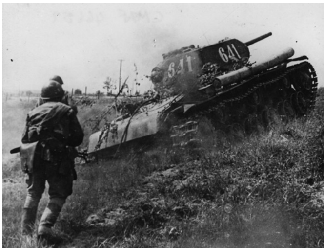
The 48th Guards Heavy Tank Regiment supported the 1st Red Banner Army's attack against the Japanese frontier defense with 21 KV-1 tanks. This KV-1 has an unditching beam attached to the tank's right side. (Courtesy of the Central Museum of the Armed Forces, Moscow, via Stavka)
