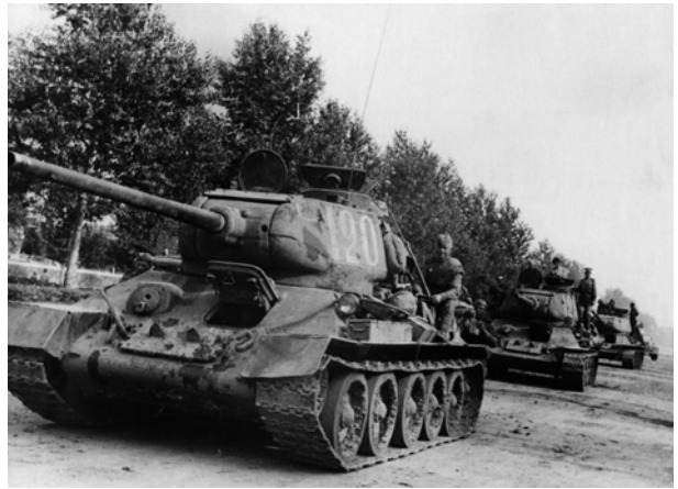
T-34-85s of the Second Far Eastern Front. The T-34-85, first fielded in 1943, had a more powerful 85mm main armament, and allowed for three crewmen in the turret. The presence of a dedicated gunner allowed the tank commander to concentrate on directing vehicle movement and fire, dramatically improving situational awareness and tank efficiency. (Sovfoto/Universal Images Group via Getty Images)
