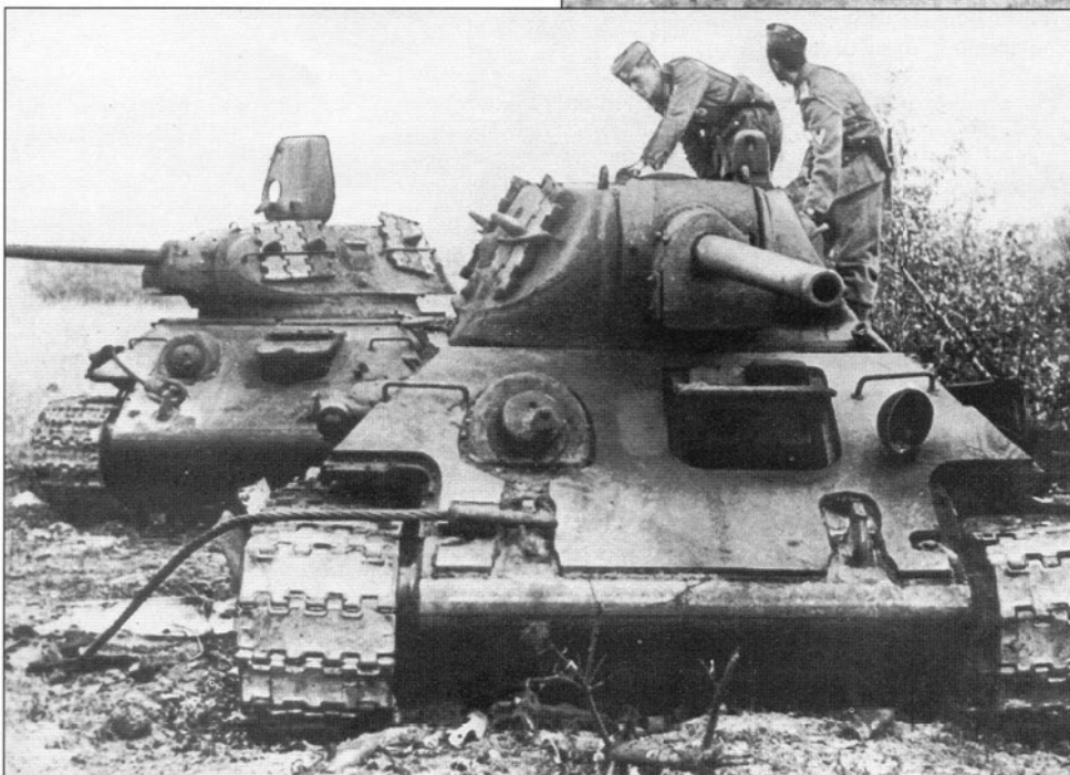
This is another example of T-34 Model 1942 tanks built at Krasnoye Sormovo No. 112 in Gorki. However, these tanks have had appliqué armor welded on to the hull front, and spare track links added for further protection. This extra armor was due to the advent of the long-barreled L/48 gun on German PzKpfw IV tanks in the summer of 1942 which could penetrate the T-34s frontal armor.
