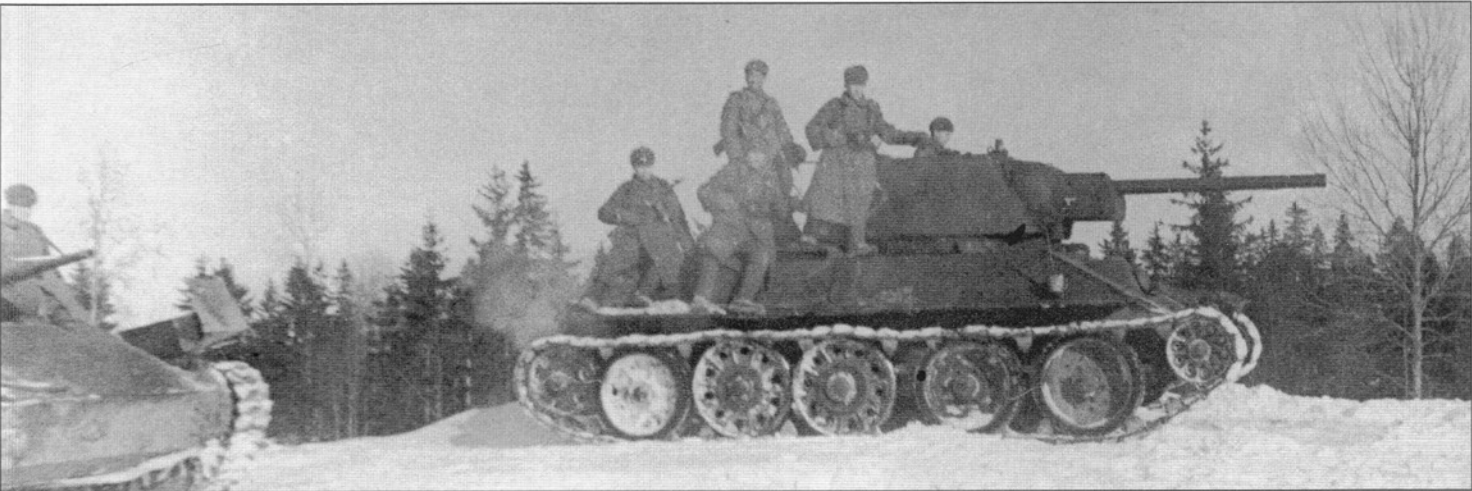
A T-34 Model 1943 and a T-70 light tank of the 144th Separate Tank Battalion during operations on 17 February 1944. These separate tank battalions were generally used to provide support to rifle divisions. Note that the T-34 has no fewer than three wheel types, probably because the first two roadwheels had been blown off by mines. (B. Vdovenko)
