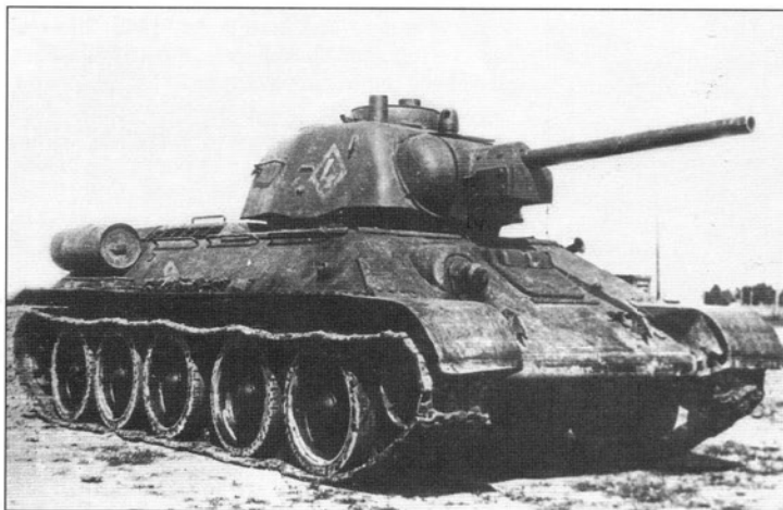
This front view of a OT-34 at Kubinka more clearly shows the ATO-42 flame-gun. The flamethrower was mounted in the hull front in place of the usual bow machine gun. The greater attention paid to flame-throwing tanks in 1943 was due to the shift in Red Army operations. As the Red Army moved to the offensive, such weapons were more necessary to overcome German fortified strongholds. (NIIBT Kubinka)
