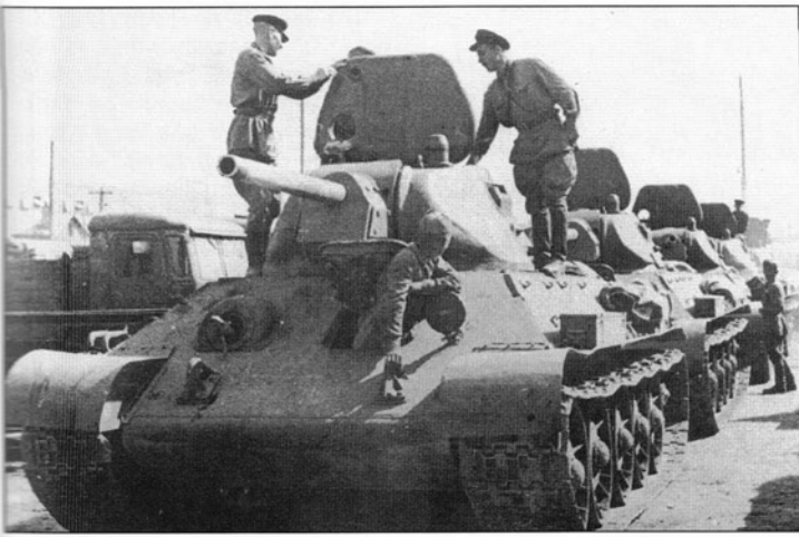
Troops of a Soviet tank brigade inspect a column of new T-34 Model 1942 tanks in the marshaling yards outside the STZ plant in Stalingrad. The STZ tanks can be distinguished by small detail features peculiar to that plant, including the interlocking glacis plate armor, and the hatchet-shaped mantlet fronts.
