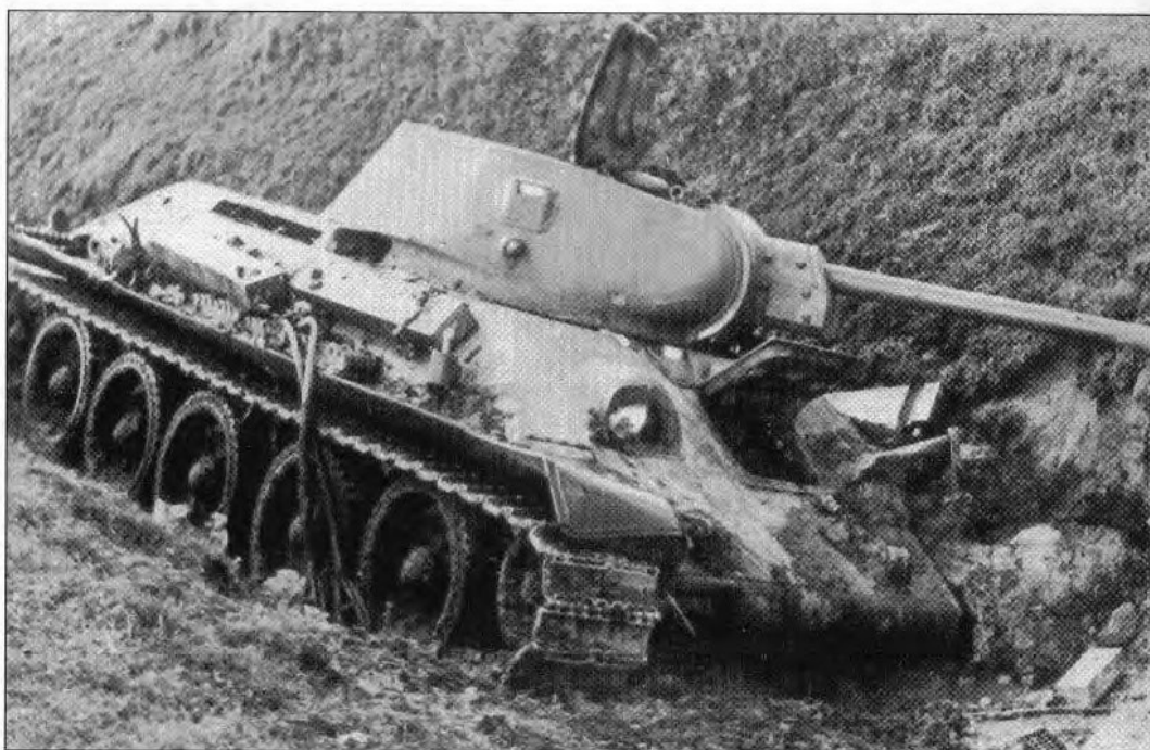
A close up of the turret of a T-34 Model 1941 which ended its service career after slipping into a bog near Mushchkotishchi during the fighting there on 1 August 1941. The vehicle has lost the periscope over the gunner's station as well as the cover over the left side armored periscope. This photo provides a good view of the early cast turret of the T-34 Model 1941. (USNA)
