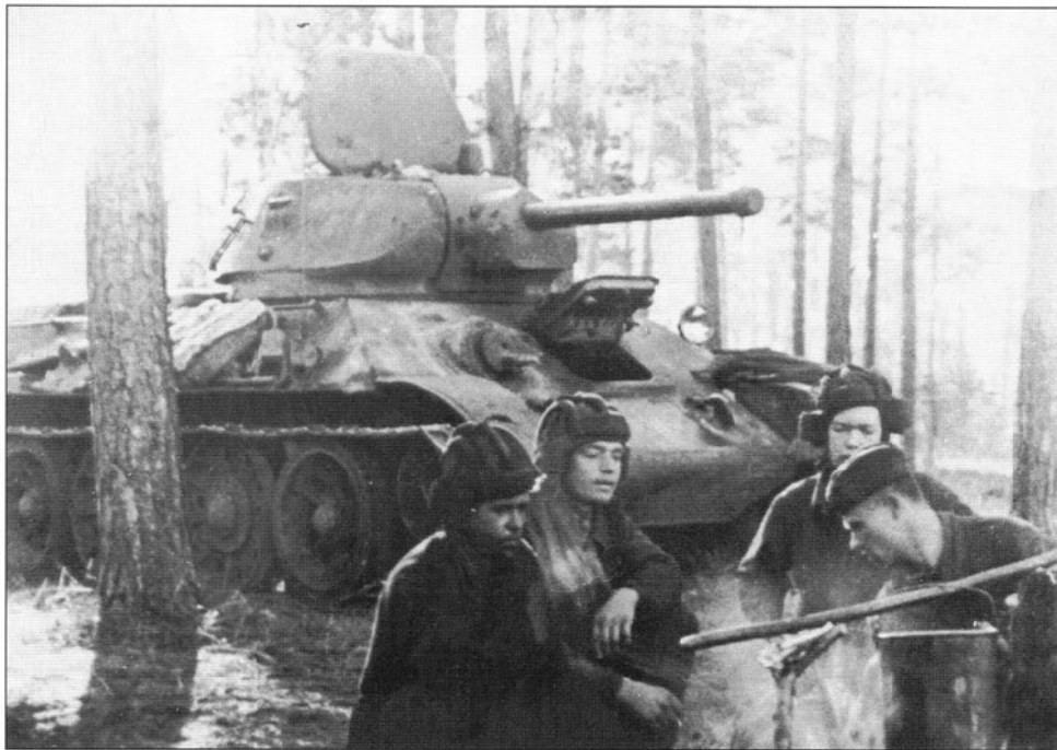
The crew of a T-34 Model 1942 with welded turret cook their meal during a lull in the fighting in 1942. This is an intermediate production Model 1942 with the improved cast turret. It has several of the mid-1942 improvements including the new PTK-5 periscope, the new hand-holds, and the armored cover over the hull machine gun.
