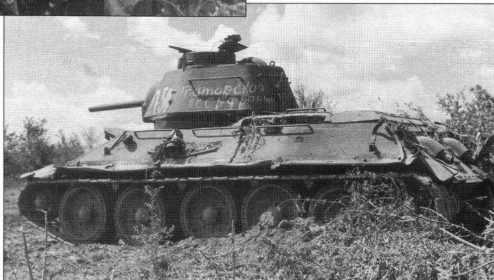
A OT-34 flamethrower tank in action in the summer of 1943. Although the flamethrower itself cannot be seen in this view, this T-34 Model 1943 can be distinguished as a flamethrower tanks by the location of the radio pot on the rear of the turret. The radio was moved from the right side of the hull front to the turret to accommodate the flamethrower equipment. The vehicle carries the legend "From the Tatar ASSR to the Front", and the vehicle tactical number is D-50.
