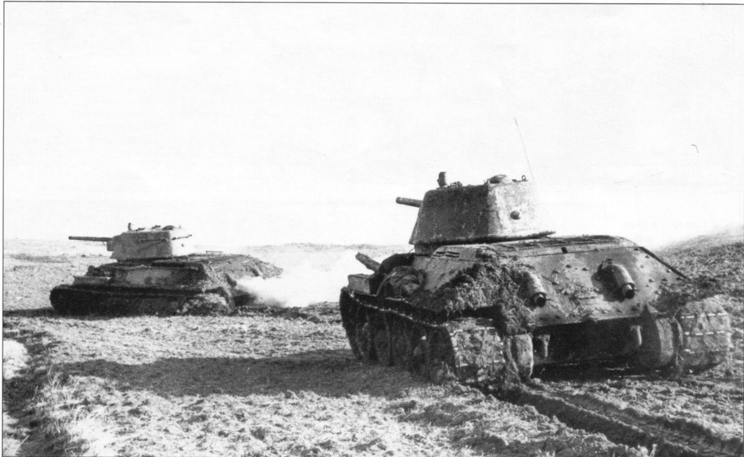
A pair of T-34 Model 1943 tanks from the same unit as the above photo. Once again, the loss of the rear fenders has caused the rear of the tank to become encrusted with mud thrown up by the tracks. The T-34 had a distinct advantage over German tanks of the period as its wide tracks enabled it to keep moving in soft soil conditions such as this which would have caused a German PzKpfw IV to become bogged down.
