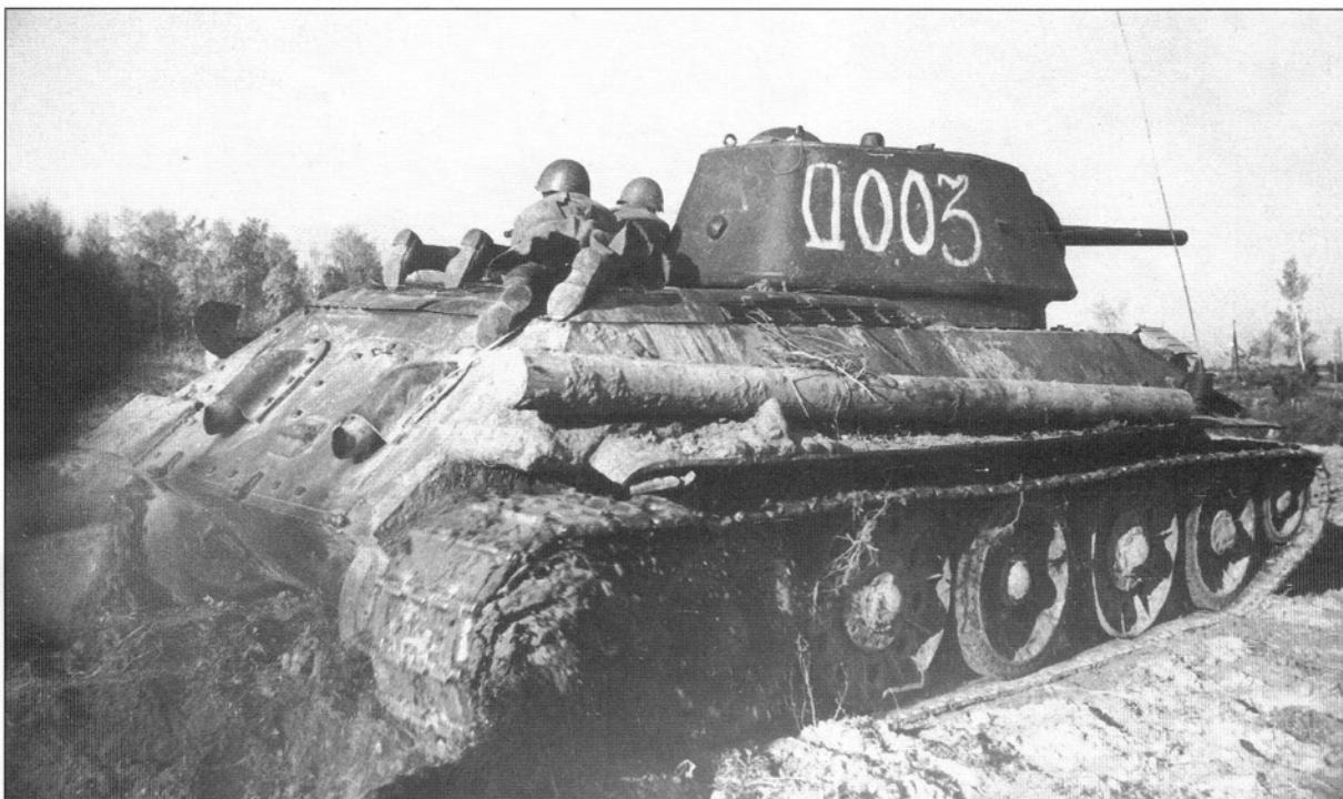
A T-34 Model 1943 of the 2nd Baltic Front moves forward towards Revel during operations in the summer of 1944. This is a relatively old vehicle with few of the 1943/44 features. The suspension is a hodge-podge of wheels, even including an old Model 1941 idler wheel. The turret tactical number is D003. (V. Grebnev)
