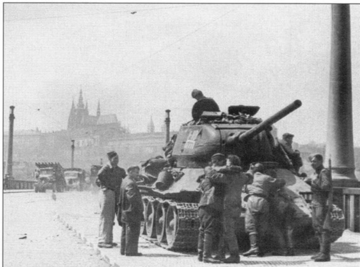
A T-34-85 of the 63rd Guards Tank Brigade rests on one of the Danube river bridges with the Hradcany castle in the background. This is a 1944 production T-34-85, evident by the original style two-piece hatch on the commander's cupola. The 1945 production version had an enlarged cupola with a one piece hatch. In the background, a BM-13 Katyusha multiple rocket launcher column moves over the bridge.
