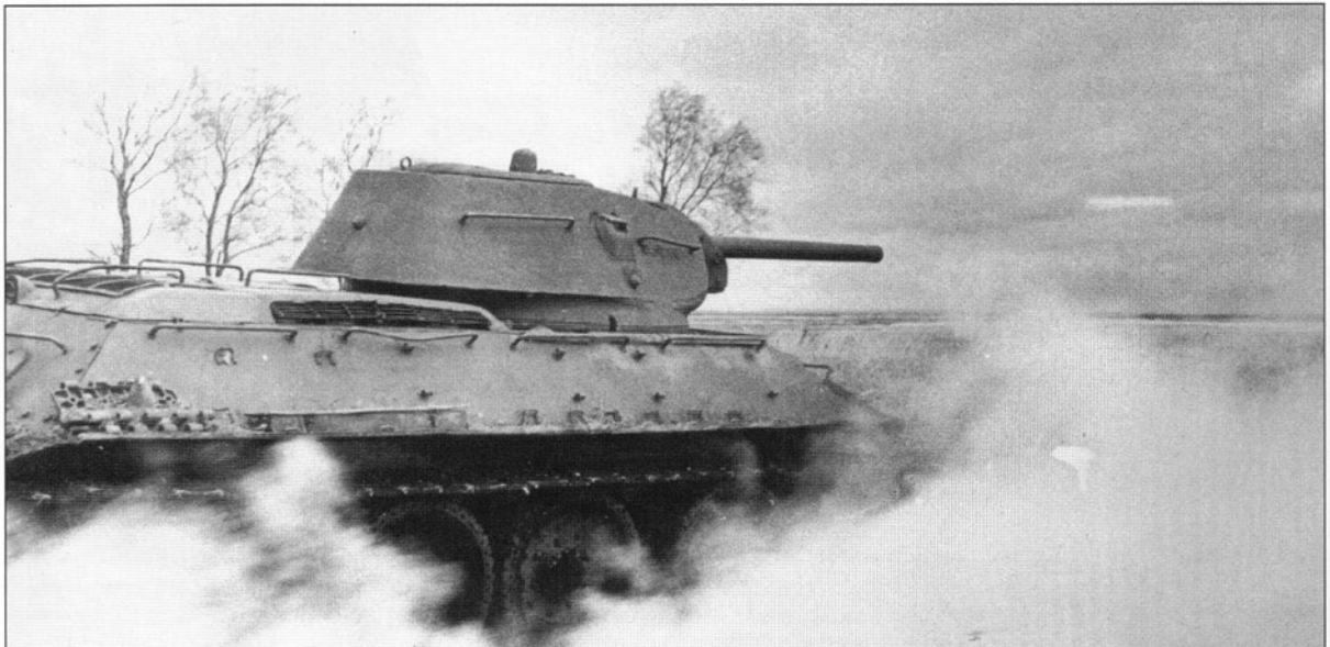
A good example of a STZ T-34 Model 1942 with welded turret. This shows most of the key distinguishing features including the Barrikady hatchet-shaped gun cover, the front turret undercut, the rear turret flat plate, the glacis (and hull rear) interlock. This vehicle has a panel of appliqué armor welded to the hull front. The slogan on the turret side is "Za Stalina!", For Stalin!
