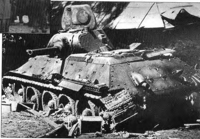
A T-34 Model 1940 knocked out during the Operation Barbarossa fighting. This is one of the late production Model 1940s, evident from the fact that the commander's periscope has been deleted from the turret hatch and plated over. The T-34 was so well armored that it was nearly impervious to German tank gun fire from the front. This tank has been knocked out by hits against its thinner rear armor.
