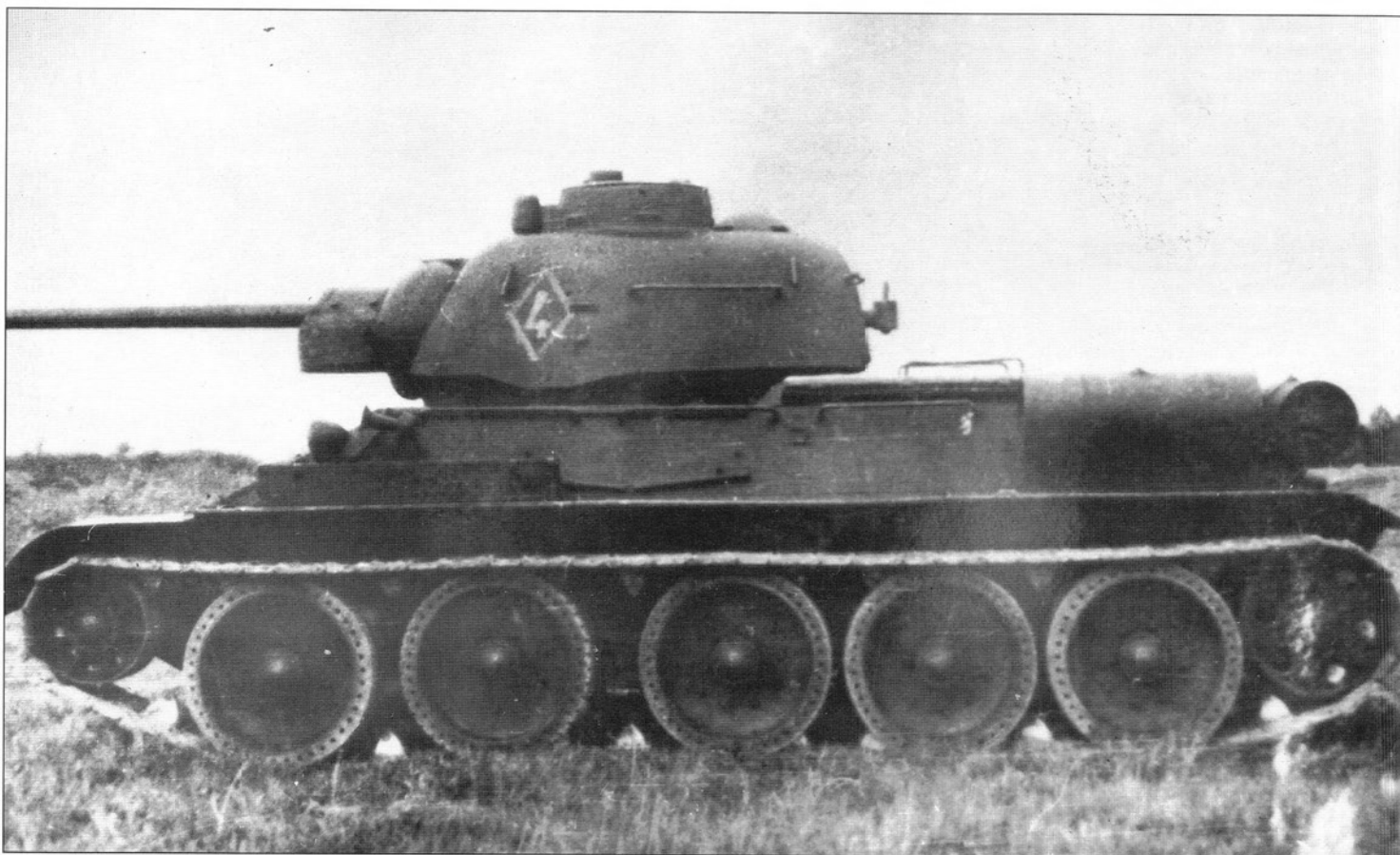
This is a side view of the OT-34 Model 1943 when it underwent trials at Kubinka in 1943. This particular example is fitted with the distinctive Uralmash turret. The repositioning of the radio pot to the turret rear is very evident in this view. The addition of the commander's cupola on the T-34 Model 1943 was another change introduced in 1943. It was originally planned to add the cupola from the KV-1S, but this was rejected as it did not have a hatch. (NIIBT Kubinka)
