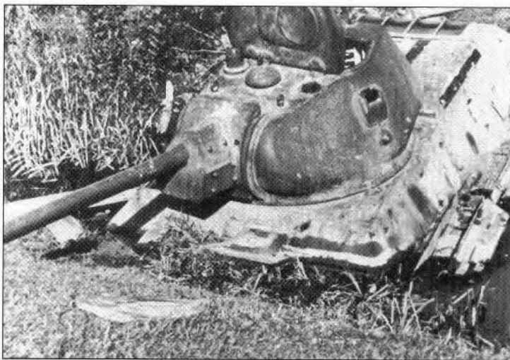
A close up of the turret of a T-34 Model 1941 which ended its service career after slipping into a bog near Mushchkotishchi during the fighting there on 1 August 1941. The vehicle has lost the periscope over the gunner's station as well as the cover over the left side armored periscope. This photo provides a good view of the early cast turret of the T-34 Model 1941. (USNA)
