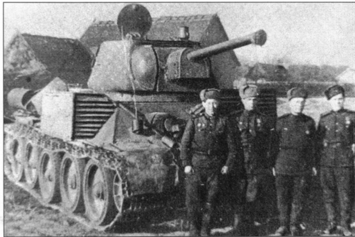
The heavy losses suffered by the Wehrmacht in 1944 made it more susceptible to desertions. This is a T-34 Model 1943 converted as a propaganda vehicle with loudspeakers in armored containers on the fender. This tank was sent near the front lines with volunteers from amongst German POWs in an effort to encourage further desertions.
