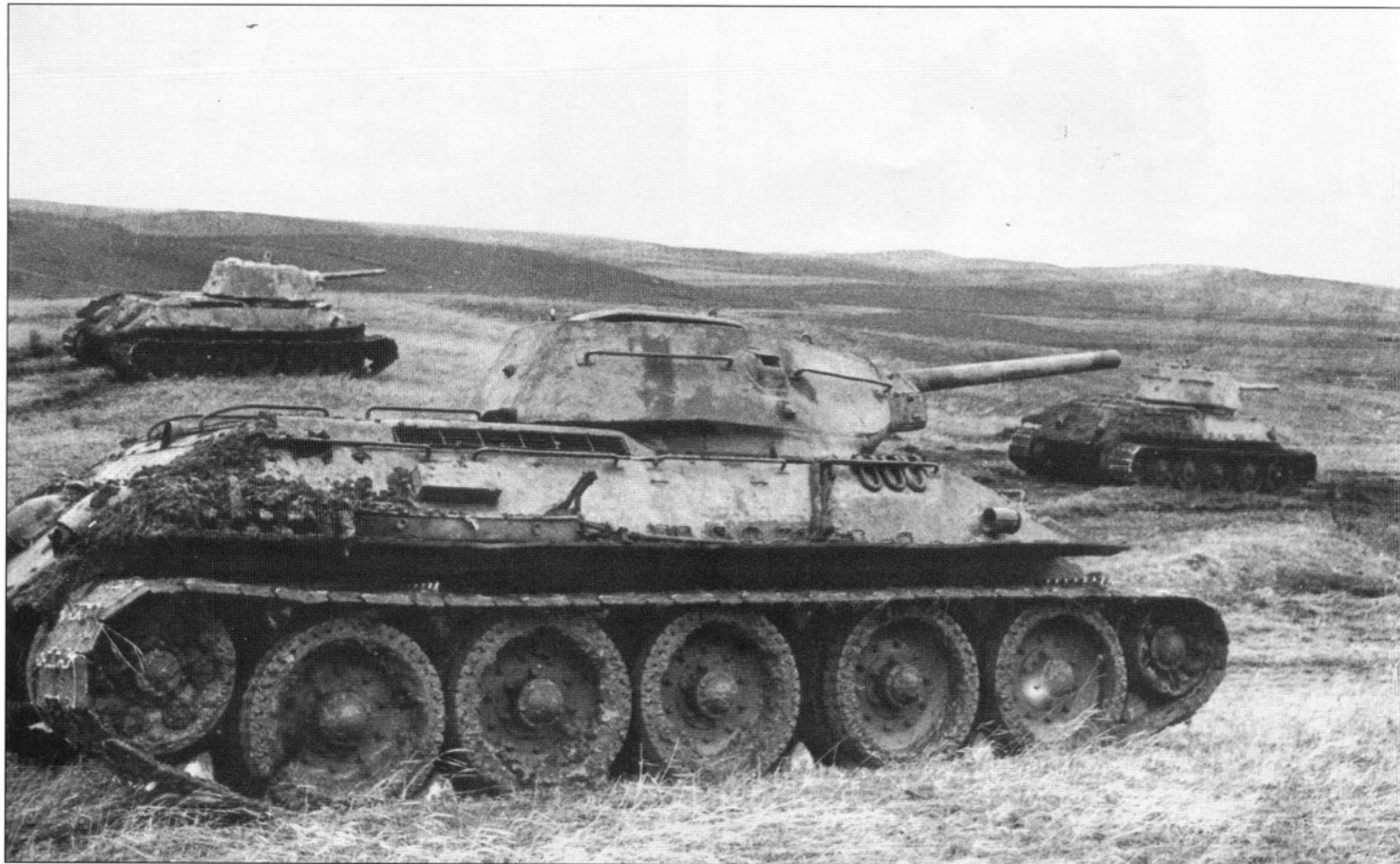
A platoon of T-34s move across the steppes in Ukraine in the autumn of 1942. The tank in the foreground is a Krasnoye Sormovo T-34 Model 1942. A look at the rear will show why tanks are fitted with fenders! In the background are two T-34 Model 1943 tanks.
