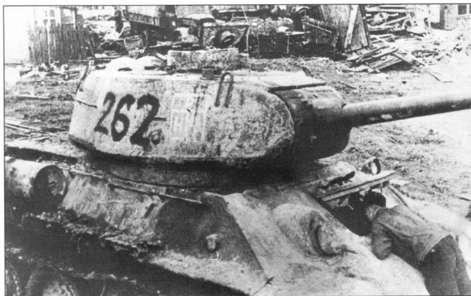
The T-34-85 was first committed to action in March-April 1944 in the fighting in southeastern Ukraine. The initial version with the expedient D-5T gun mounting was quickly supplanted by the standard version with the ZiS-S-53 85mm gun as seen here. The original vehicles, manufactured in April 1944, still had the unusual upside-down "U" hooks on the turret, but the turret had several new features. The new gun can be distinguished by the different type of collar, and the commander's cupola has been pushed back further on the turret roof due to the introduction of a new articulated gunner's telescopic sight.
