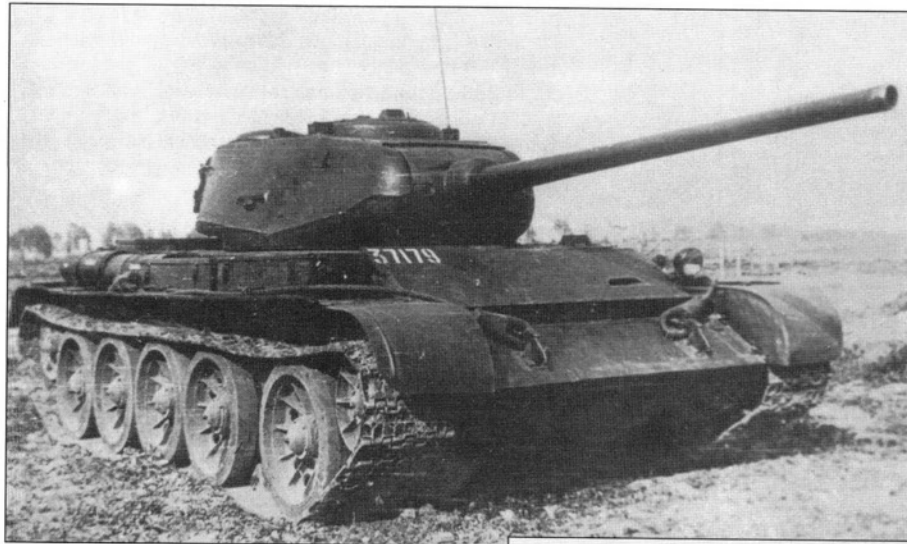
This is the third prototype of the T-44 at Kubinka in the summer of 1944. On this vehicle, the driver's hatch has been moved entirely to the top of the hull roof and the turret moved back on the hull slightly to accommodate it. Later in 1944, the designers also investigated upgunned versions, the T-44-100 with the D-5T 100mm gun, and the T-44-122 with the 122mm D-25T gun. (NIIBT Kubinka)
