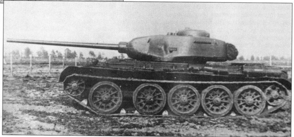
This is a side view of the second prototype of the T-44. Although the turret is similar to that on the T-34-85, it is by no means identical as is evident in this view. A total of 965 were built in 1944-45. The first three tank units were formed on the T-44 on 15 September 1944, the 6th Guards, 33rd Guards, and 63rd Guards Tank Brigades. However, units were organized to train troops on the new tanks. Due to prolonged teething problems with the tanks as well as a desire to keep the new design secret, no T-44s were used in combat in 1945. (NIIBT Kubinka)
