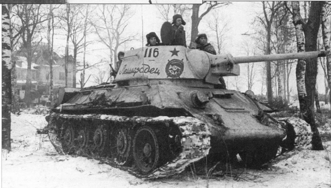
A good example of the style of appliqué armor fitted to tanks on the Leningrad Front by rebuilding factories in the city. These T-34 Model 1942s are moving forward on 21 January 1944 during efforts by the 2nd Shock Army to finally lift the siege of the city. There were still significant numbers of old tanks in the Leningrad area, including old model T-34s such as these, T-28s and BT-7s as late as 1944 due to the isolation of the city.
