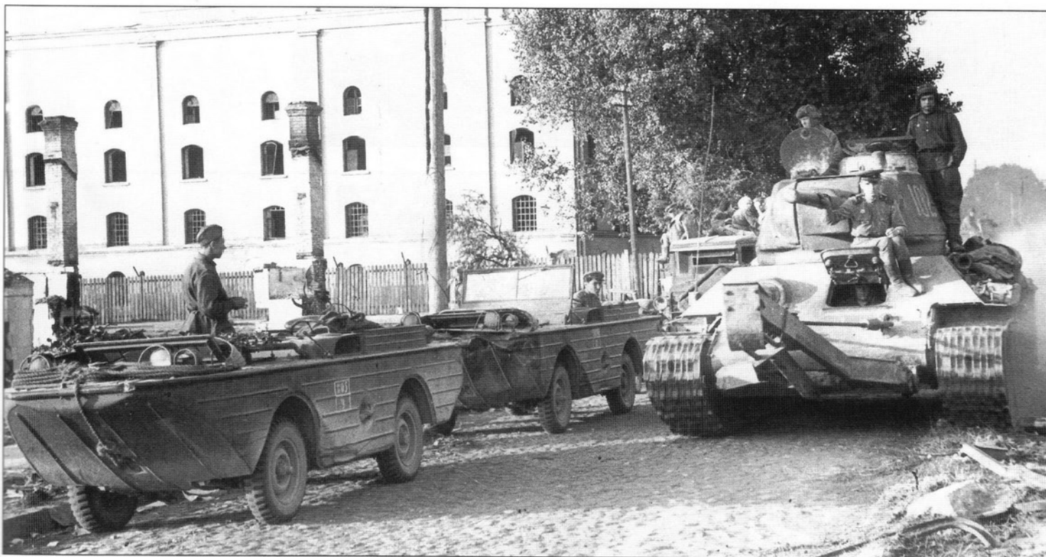
A T-34 Model 1943 passes by a column of GPA (amphibious jeeps) during the 3rd Baltic Front's liberation of the Lithuanian capital of Vilnius on 13 July 1944. This tank is fitted out as a PT-34 mine roller. It has the yoke for the mine rollers attached, but the wheels themselves are not fitted. Usually, the tanks moved into the assembly area without the roller wheels and they were carried separately on trucks until the needed to be attached. The amphibious jeeps were generally used by Soviet razvedchik scout units to secure small bridgeheads in advance of the main body of troops. —
