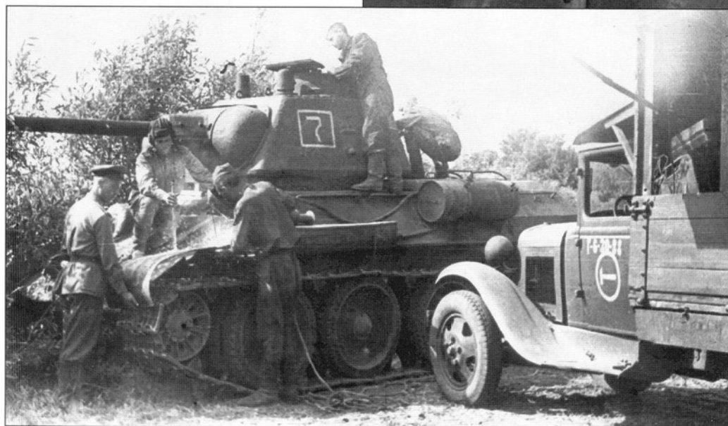
A T-34 Model 1943 tank of the 13th Guards Mechanized Brigade, 4th Guards Mechanized Corps during operations on the 3rd Ukrainian Front in Romania in the late summer of 1944. The tank is undergoing repairs from a mobile repair vehicle. It would appear that the repair team is welding on the front mud guard.
