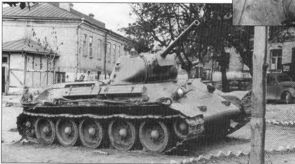
A detailed close-up of a T-34 Model 1940 knocked out during the 1941 fighting and sent back to Germany for technical evaluation. This provides a good view of the early cast turret and other details. For example, this tank is fitted with the turret hatch periscope, rarely seen in place, though the upper cover has been blown off presumably when the tank was hit. It is missing several other small parts.
