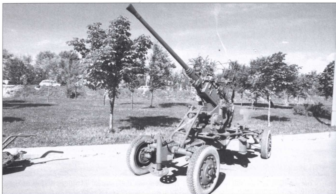
Probably the most familiar Soviet anti-aircraft gun of the Second World War was the 37mm 61-K Model 1939 based on the imported Swedish 40mm Bofors gun. It bears a strong family resemblance to its Swedish ancestor and was used throughout the war by Soviet Army air defence units. (S. Zaloga)
