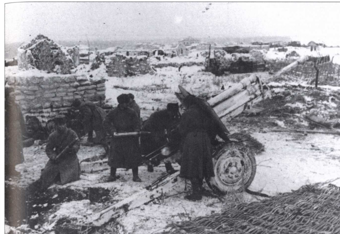
A standard weapon of the Soviet divisional artillery was the 76mm divisional gun. This particular example is an F-22 USV , an interim design of the late 1930s which preceded the wartime ZiS-3 type. This category of weapon is frequently misunderstood in Western accounts as an anti-tank weapon, partly because the Germans used captured examples in this role. This weapon is seen in use during the Stalingrad fighting in 1942.
