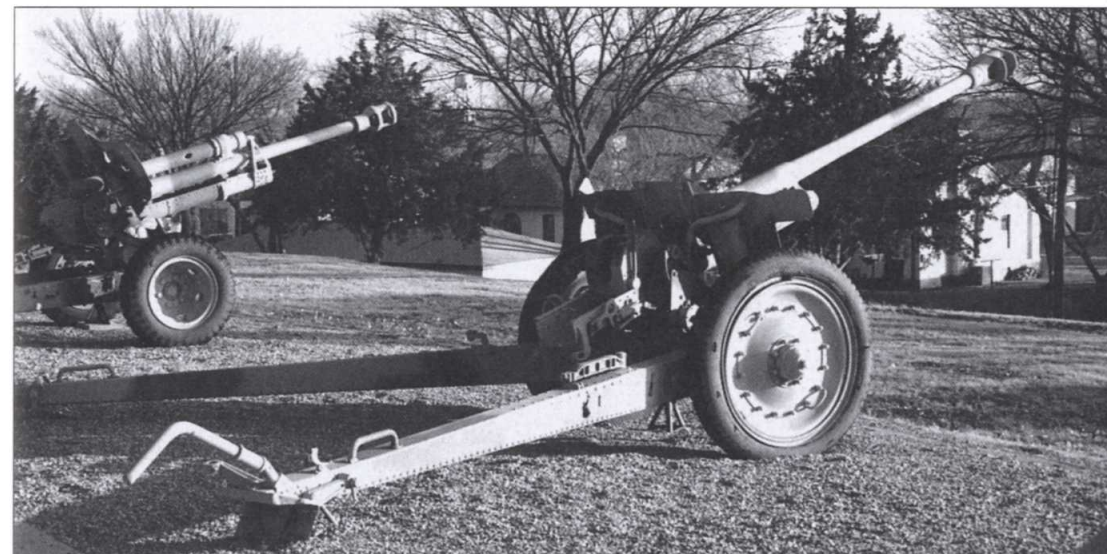
The first modern divisional gun in Red Army service was the 76mm F-22 Model 1936. Although a fine weapon, it was expensive and quite heavy. The German Wehrmacht captured the F-22 in large numbers and used them in service as anti-tank guns until their own 75mm PaK 40 became available. Indeed the gun here is a former German weapon, captured by the US Army in North Africa. The German version was distinguished by a lower splinter shield and a muzzle brake. (S. Zaloga)
