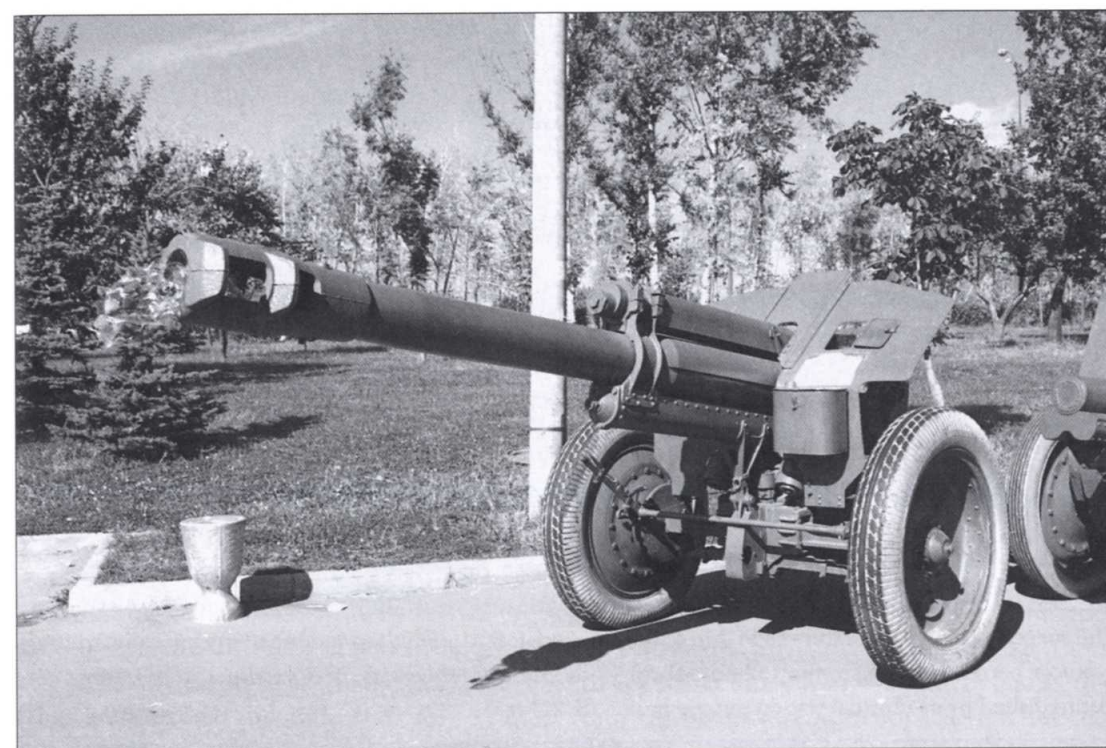
To replace the expensive M-10 Model 1938 field howitzer, the D-1 Model 1943 was developed, using the carriage of the widely used M-30 122mm howitzer. Although similar in appearance, it can be distinguished by its prominent muzzle brake. (S. Zaloga)
