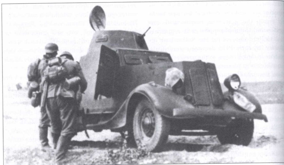
The Red Army built large numbers of armoured cars before the war, primarily for reconnaissance roles. The BA-20 was the latest model in the light armoured car category and was based on a standard civilian automobile chassis. Here, a captured example is examined by German troops in 1941.
