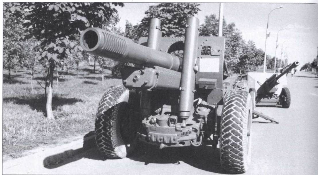
The success of the A-19 122mm field gun led to the decision to adapt it to mount a larger 152mm gun-howitzer barrel, resulting in the 152mm ML-20 Model 1937 gun-howitzer. This version can be easily distinguished by its unusual slatted muzzle brake. (S. Zaloga)
