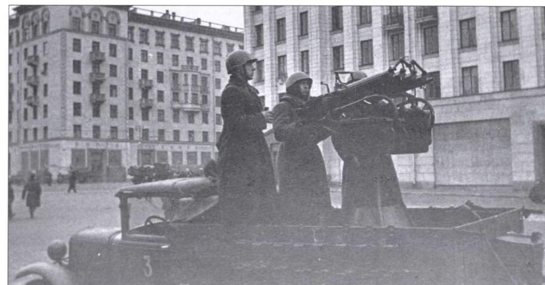
One of the standard anti-aircraft weapons of the Red Army was the Tokarev 4M Model 1931 quadruple anti-aircraft machine gun mounting. This consisted of four Maxim Model 1910 machine guns on a heavy pedestal mount with associated ammunition and water-cooling tank. Due to its size and weight, it was usually mounted on a lorry, such as the GAZ-AAA seen here, or emplaced in a fixed site.
