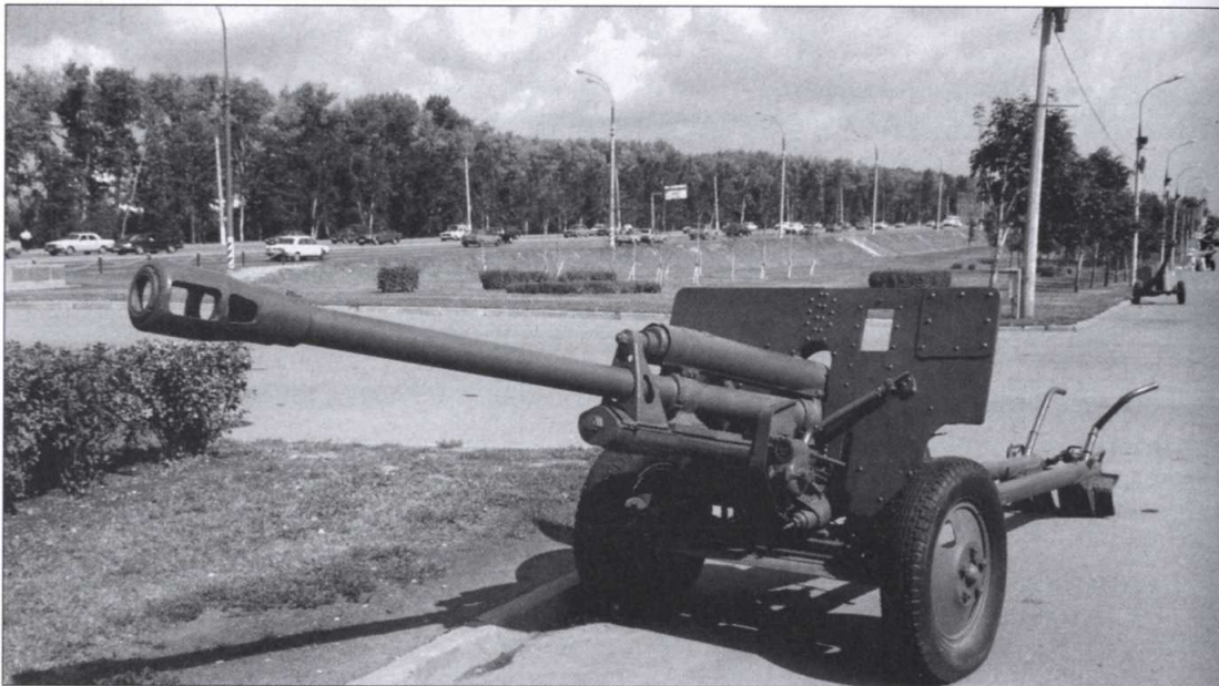
Neither the F-22 nor the F-22 USV were sufficiently light and simple, and a third design, the ZiS-3, followed in 1941, based on the carriage of the short-lived ZiS-2 57mm anti-tank gun. This became the standard divisional gun of the Red Army after 1942 and was so successful that it was still being exported in the 1980s. (S. Zaloga)
