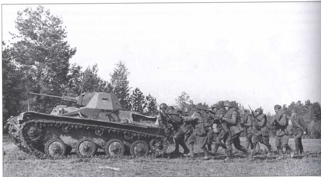
Soviet automotive factories could not produce designs as large and heavy as the T-34 and so instead were diverted to manufacture light tanks such as the T-60. Armed only with a 20mm gun, the T-60 proved inadequate in combat. In 1942 it was replaced by the slightly larger T-70 light tank, armed with a better 45mm gun.
