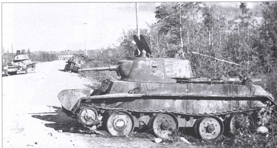
The BT-7 fast tank was intended for use by the large mechanized formations to conduct deep operations, and was comparable to British cruiser tanks. Although well armed for its day, its thin armour proved a liability and thousands were lost in 1941, such as this example destroyed in combat with the Finnish Army on the Karelian peninsula in 1941. (Esa Muikku)
