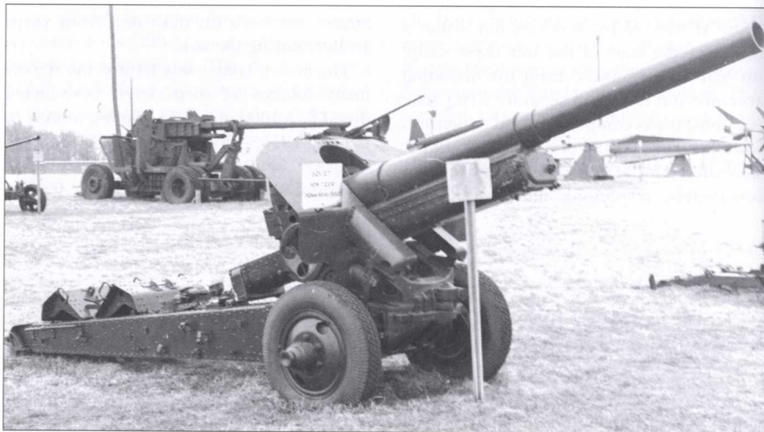
The Red Army fielded a fine new 152mm field howitzer, the M-10 Model 1938, before the outbreak of the war. Although well regarded, it was complicated and expensive to manufacture and production ended after the outbreak of the war. (S. Zaloga)
