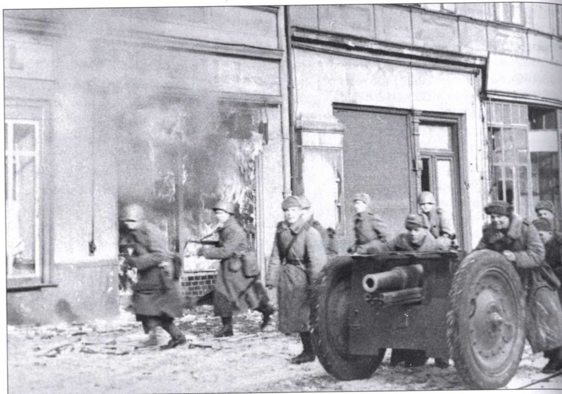
Another common Soviet artillery weapon was the 76mm Model 1927/39 regimental gun. This was a modernized version of the old Tsarist 3in gun, and provided the infantry with a handy source of direct-fire support. Here, one is being manhandled into position during streetfighting in Gleiwitz, Germany, in 1945.
