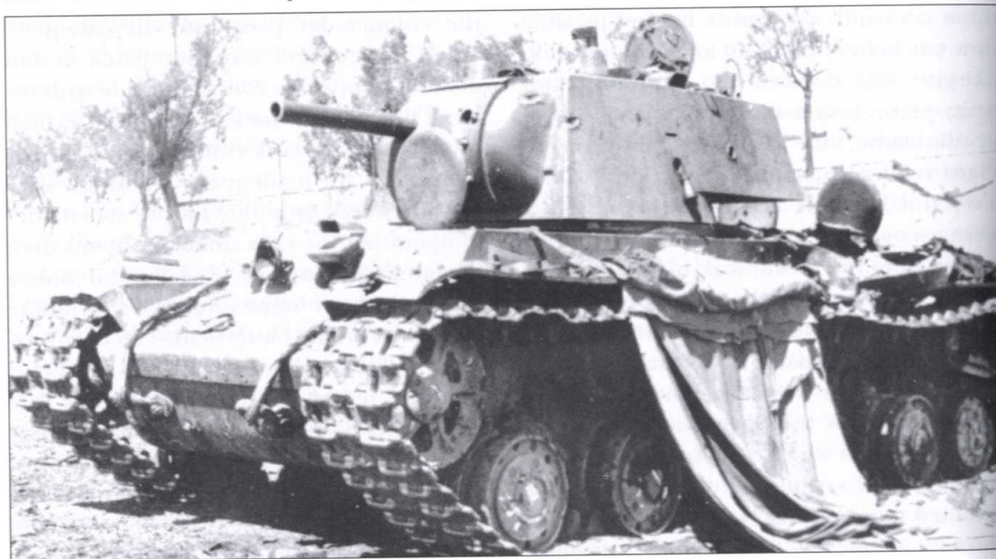
No weapon terrorized German infantry in 1941 more than the KV-1 heavy tank. Impervious to the standard German 37mm anti-tank gun, there were several recorded instances of the KV simply running over and crushing Wehrmacht guns. Numerous hits can be seen on this KV-1 of the 6th Mechanized Corps, knocked out finally by an 88mm gun near Zelva, Lithuania, in July 1941. The Achilles heel of the design was a balky transmission and powertrain, exacerbated by poor crew training.
