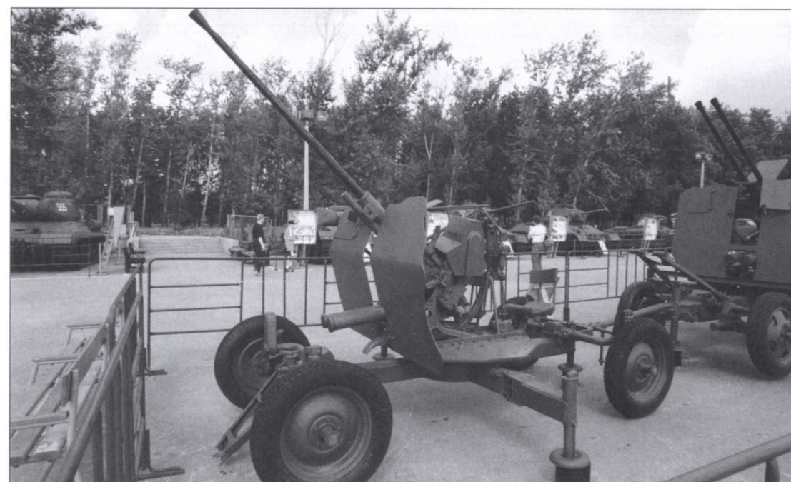
Soviet light anti-aircraft guns were heavily influenced by imported Swedish Bofors designs. The 25mm 72-K Model 1940 was a standard design which entered service in late 1941. It is not well known outside the Soviet Union as it was intended for use by national air defence forces, not for tactical Army air defence, and so was not often captured by the Germans. (S. Zaloga)
