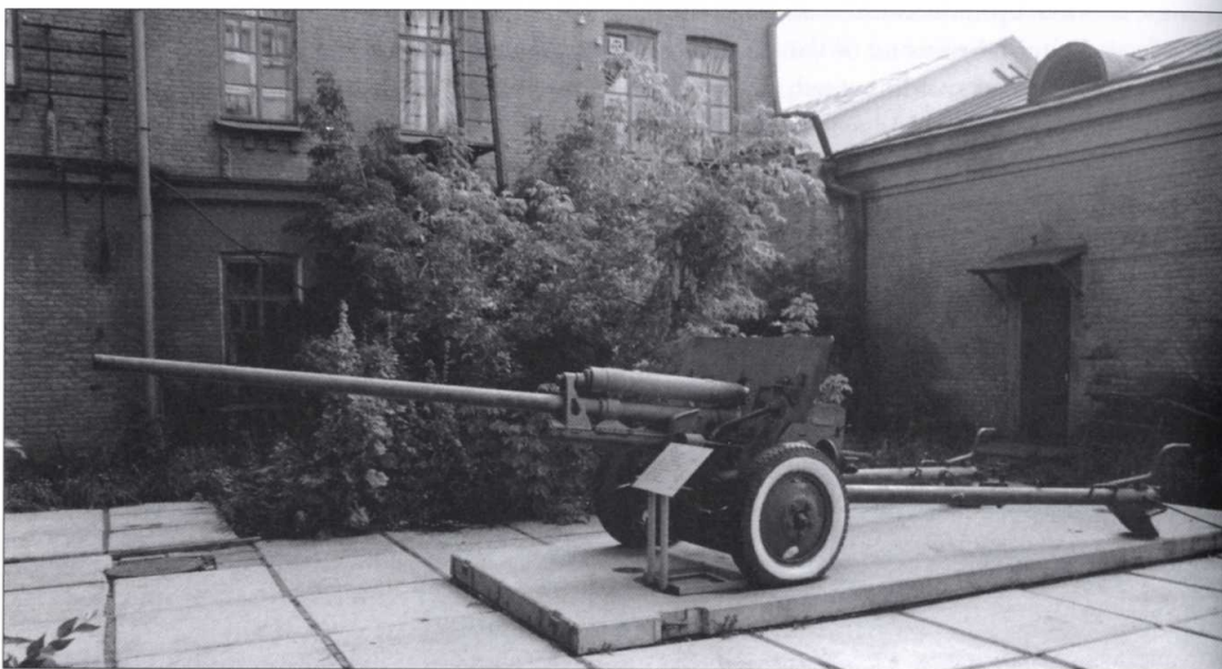
The Red Army introduced the excellent ZiS-2 57mm anti-tank gun into service in 1941 but its production was abruptly cancelled by Stalin's cronies owing to intelligence mistakes about German tank armour. Production was revived in 1943 to deal with the heavier German tank armour. The 57mm Model 1943, as seen here, used the same tubular trails as the related ZiS-3 76mm divisional gun, while the Model 1941 used rectangular trails. (S. Zaloga)
