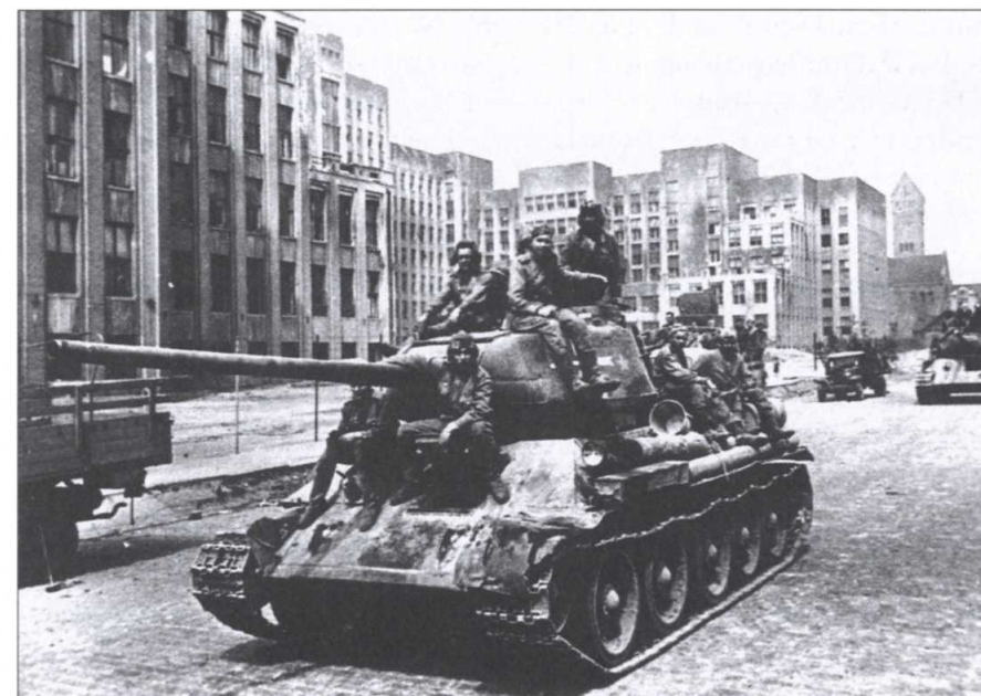
Kursk was a painful reminder of how far Soviet tank technology had slipped behind German due to its concentration on quantity over quality. As a result of the appearance of the German Panther tank, Soviet tank designers were forced rapidly to develop a better armed version of the T-34, fitted with an 85mm gun. The resulting T-34-85 tank entered combat in the spring 1944 offensives and is seen here during the liberation of Minsk at the conclusion of Operation Bagration in Belorussia in the summer of 1944.
