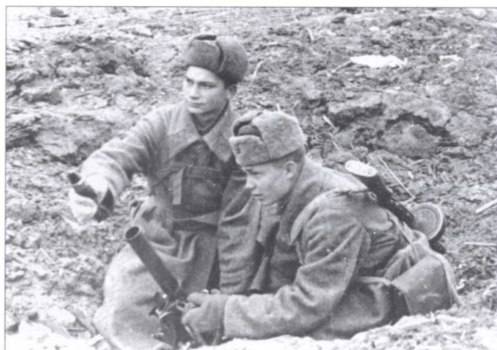
The 50-PM 41 (50mm infantry mortar Model 1941) was an attempt to simplify the production of light infantry mortars; it dispensed with the bipod, using a simple yoke instead, and could hurl a 1.8lb mortar bomb about 875 yd.
