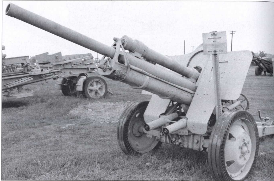
The F-22 was quickly followed into production by the F-22 USV Model 1939 which was an attempt to lighten and simplify it. It was the standard Red Army divisional gun at the outset of the war. (S. Zaloga)
