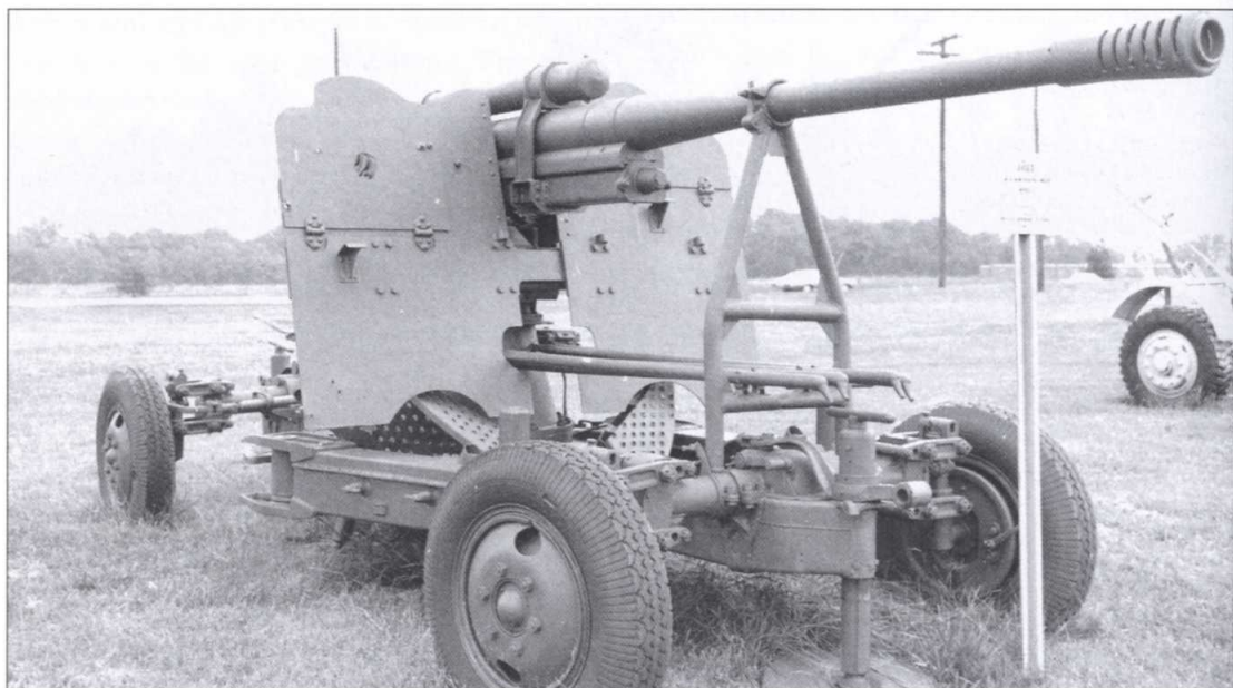
The 85mm Model 1939 anti-aircraft gun was intended primarily for national air defence but was sometimes seen in front-line service. In 1943 the Red Army formed a number of expedient anti-tank brigades armed with the weapon to deal with the new German heavy tanks until a more suitable towed anti-tank gun became available. Unlike the Wehrmacht and its legendary 88mm gun, the Red Army did not use this weapon widely for tank fighting. (S. Zaloga)
