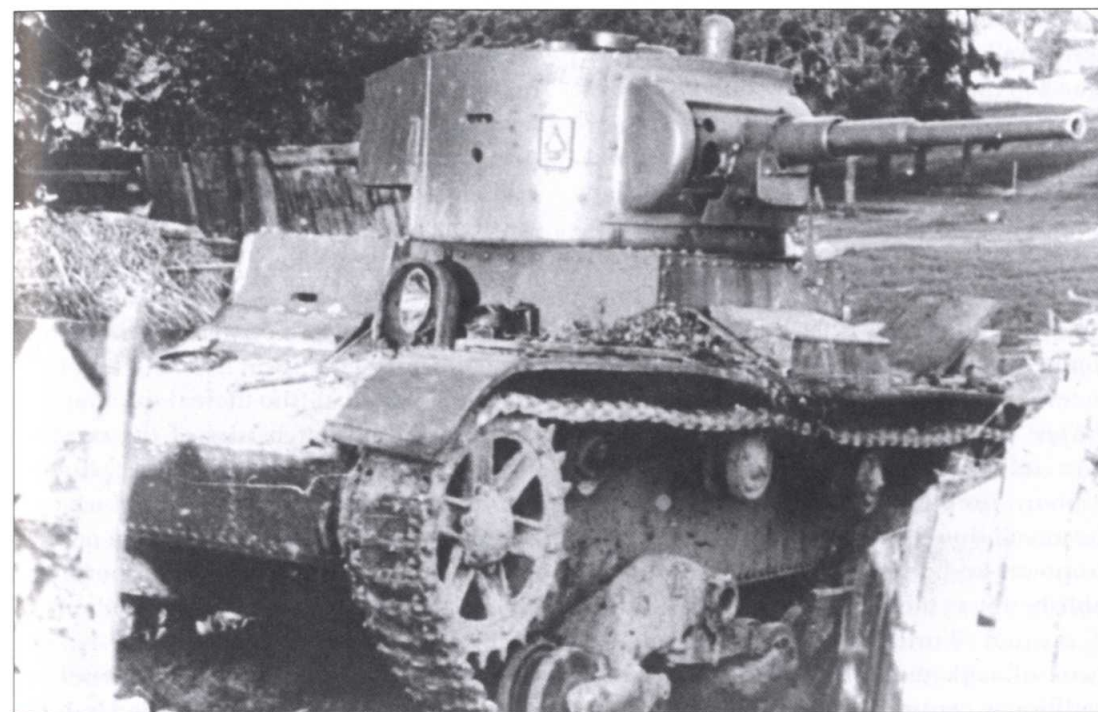
The most common Soviet tank in 1941 was the T-26 Model 1933 light tank, a derivative of the British Vickers 6-ton export tank. It was intended primarily for infantry support and had a distinguished combat record during the Spanish Civil War. But by 1941 its poor mechanical state and thin armour doomed it to extinction.
