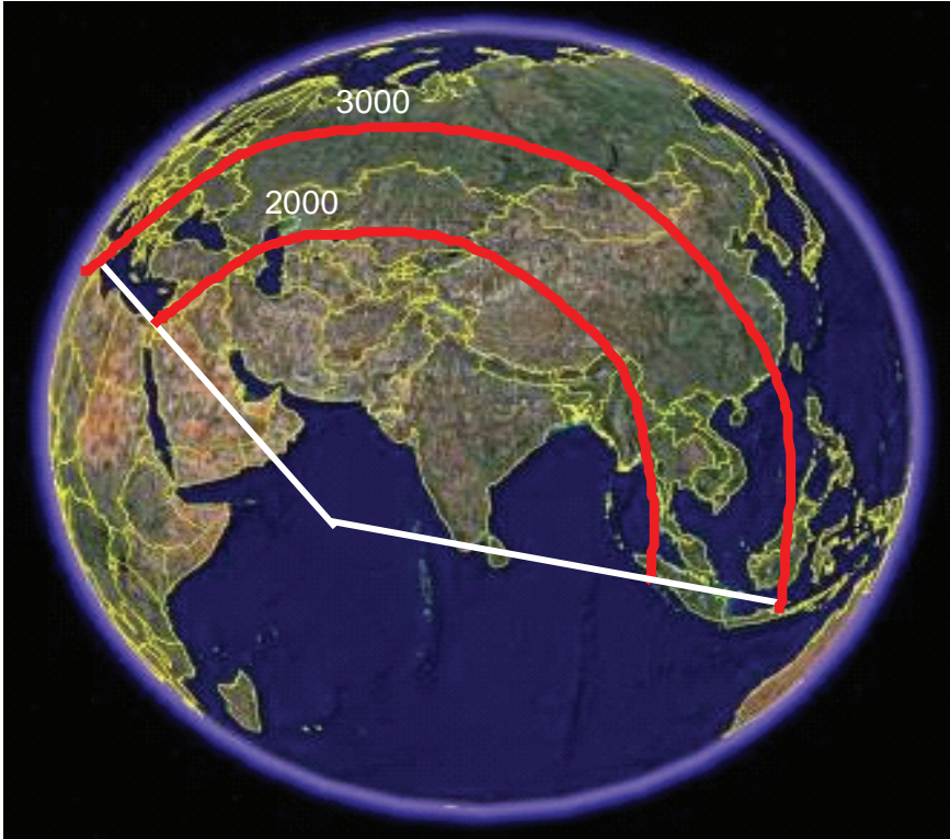
FIGURE 4-6 Sample ranges (in nautical miles) from a notional nuclear-powered guided missile submarine (SSGN) launch location in the Arabian Sea illustrating the need for a conventional prompt global strike range capability of 2,500 to 3,500 nmi when launched from an SSGN.
