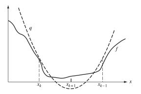
Fig. 8.5 False position for minimization
