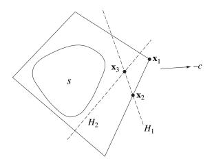
Fig. 14.7 Cutting plane method
