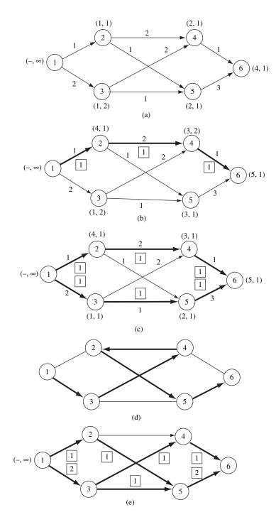
Fig. 6.6 Example of maximal flow problem
