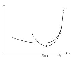
Fig. 8.3 Newton's method for minimization
