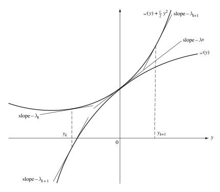
Fig. 14.5 Primal function and augmented Lagrangian
