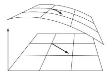
Fig. 12.11 Induced coordinate system
