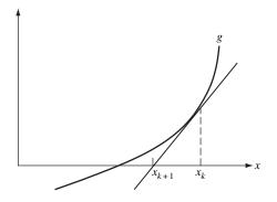
Fig. 8.4 Newton's method for solving equations
