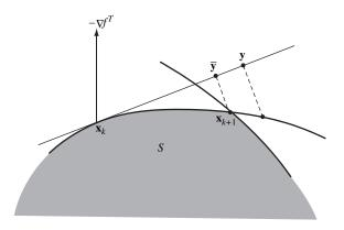
Fig. 12.7 Interpolation to obtain feasible point
