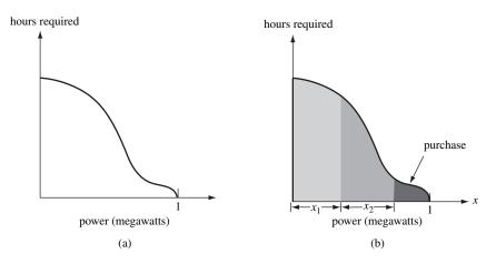
Fig. 7.2 Power requirements curve
