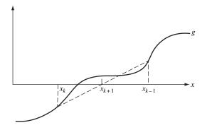
Fig. 8.6 False position for solving equations
