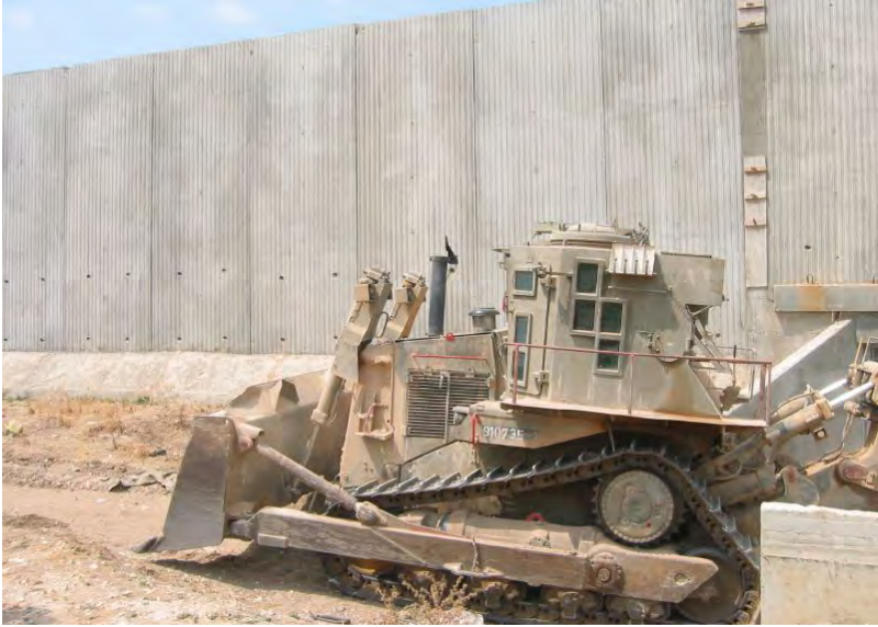
1/// Israeli customized bulldozer Caterpillar D9 along the Barrier /// Photograph by Joe Skillet
