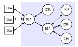
The data stored in X.500 servers is organized in a tree structure with named nodes, as in the case of the other name servers discussed in this chapter, but in X.500 a wide range of attributes are stored at each node in the tree, and access is possible not just by name but also by searching for entries with any required combination of attributes.
