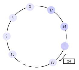
*Note:* The election was started by process 17. The highest process identifier encountered so far is 24. Participant processes are shown in a darker tint.
