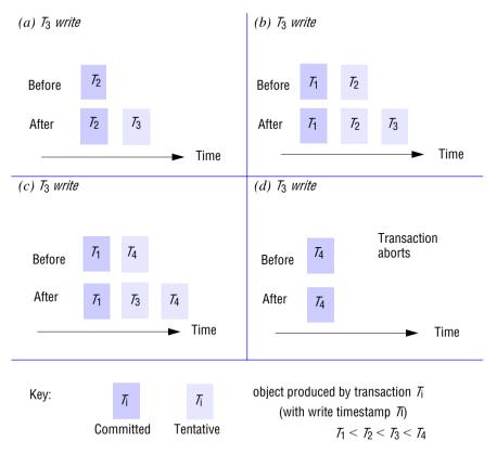
Timestamp ordering write rule: By combining rules 1 and 2 we get the following rule for deciding whether to accept a *write* operation requested by transaction  $T_c$  on object D:
