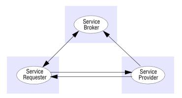
service requester and service broker (a service that matches services provided to those requested), as shown in Figure 2.11. This brokerage pattern is replicated in many areas of distributed systems, for example with the registry in Java RMI and the naming service in CORBA (as discussed in Chapters 5 and 8, respectively).
