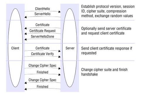
giving an error indication if it has none that match). At this stage they also agree on a (optional) compression method and a random start value for CBC block encryption functions (see Section 11.3).
