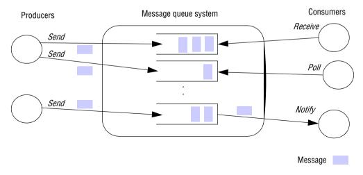
content is serialized using any of the standard approaches described in Section 4.3; that is, marshalled data types, object serialization or XML structured messages. Message sizes are configurable and can be very large – for example, on the order of a 100 Mbytes Given the fact that message bodies are opaque, message selection is normally expressed through predicates defined over the metadata.
