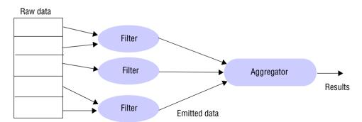
**Figure 21.20** The overall execution of a Sawzall program
