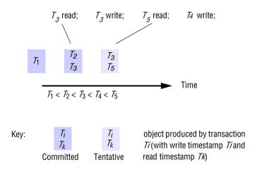
Multiversion timestamp ordering write rule: As any potentially conflicting *read* operation will have been directed to the most recent version of an object, the server inspects the version  $D_{maxEarlier}$  with the maximum write timestamp less than or equal to  $T_c$ . We have the following rule for performing a *write* operation requested by transaction  $T_c$  on object D:
