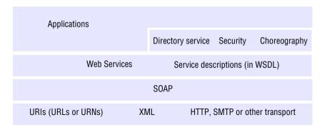
in XML. SOAP is used to encapsulate these messages and transmit them over HTTP or another protocol, for example, TCP or SMTP. A web service deploys service descriptions to specify the interface and other aspects of the service for the benefit of potential clients.
