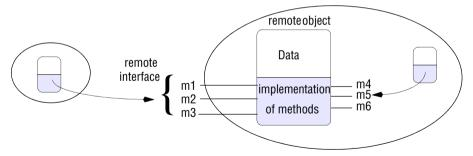
Remote interfaces: The class of a remote object implements the methods of its remote interface, for example as public instance methods in Java. Objects in other processes can invoke only the methods that belong to its remote interface, as shown in Figure 5.13. Local objects can invoke the methods in the remote interface as well as other methods implemented by a remote object. Note that remote interfaces, like all interfaces, do not have constructors.
