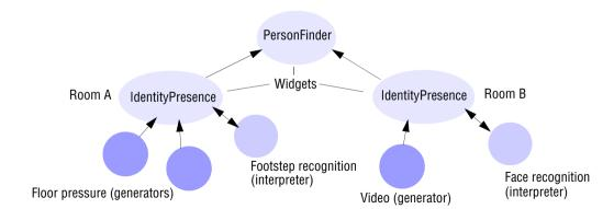
**Figure 19.6** A *PersonFinder* widget constructed using *IdentityPresence* widgets
