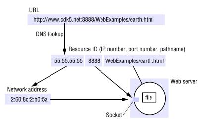
Figure 13.1 Composed naming domains used to access a resource from a URL
