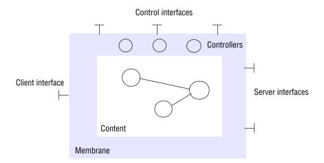
visible to components within the content part, or *external* and hence visible to any other components. This structure is illustrated in Figure 8.17.
