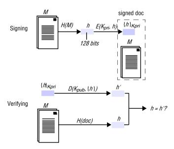
verified by a principal that subsequently receives the document to check that it was originated by A and that its contents, M, have not subsequently been altered.
