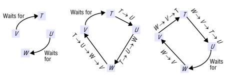
**Transaction priorities** • In the above algorithm, every transaction involved in a deadlock cycle can cause deadlock detection to be initiated. The effect of several transactions in a cycle initiating deadlock detection is that detection may happen at several different servers in the cycle, with the result that more than one transaction in the cycle is aborted.
