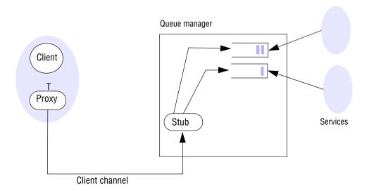
whereby MQI commands are issued on the proxy and then sent transparently to the queue manager for execution using RPC. An example of such a configuration is shown in Figure 6.15. In this configuration, a client application is sending messages to a remote queue manager and multiple services (on the same machine as the server) are then consuming the incoming messages.
