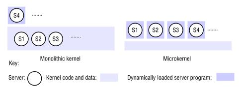
Ideally, the kernel would provide only the most basic mechanisms upon which the general resource management tasks at a node are carried out. Server modules would be dynamically loaded as required, to implement the required resource management policies for the currently running applications.
