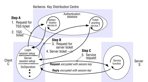
Figure 11.15 System architecture of Kerberos
