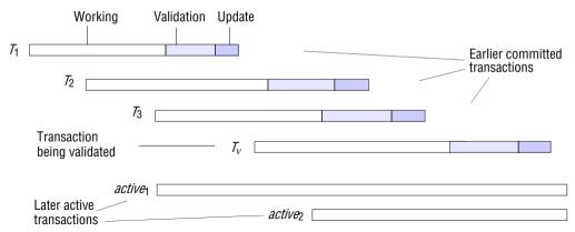
implemented outside the critical section, but it is essential that the assignment of transaction numbers is performed sequentially. We note that at any instant, the current transaction number is like a pseudo-clock that ticks whenever a transaction completes successfully.
