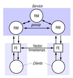
to record the version of the replicated data that has been observed by the client. (See Section 14.4 for a definition of vector timestamp merging.)
