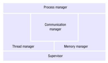
Figure 7.2 shows the core OS functionality that we shall be concerned with: process and thread management, memory management and communication between processes on the same computer (horizontal divisions in the figure denote dependencies). The kernel supplies much of this functionality – all of it in the case of some operating systems.
