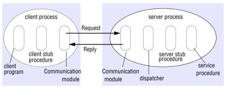
then unmarshals the arguments in the request message, calls the corresponding service procedure and marshals the return values for the reply message. The service procedures implement the procedures in the service interface. The client and server stub procedures and the dispatcher can be generated automatically by an interface compiler from the interface definition of the service.
