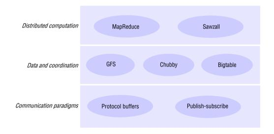
**Google infrastructure** • The system is constructed as a set of distributed services offering core functionality to developers (see Figure 21.6). This set of services naturally partitions into the following subsets:
