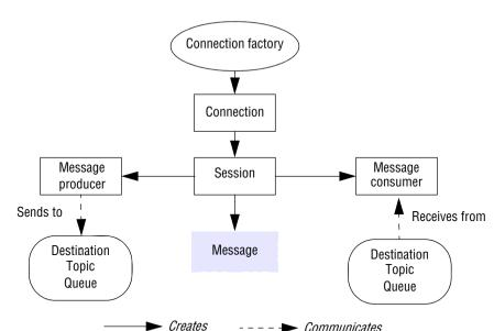
Figure 6.16 The programming model offered by JMS
