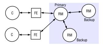
This system obviously implements linearizability if the primary is correct, since the primary sequences all the operations upon the shared objects. If the primary fails, then the system retains linearizability if a single backup becomes the new primary and if the new system configuration takes over exactly where the last left off. That is if:
