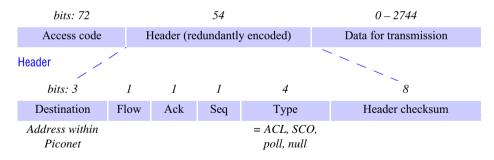
SCO packets (e.g., for voice data) have a 240-bit payload containing 80 bits of data triplicated, filling exactly one timeslot.
