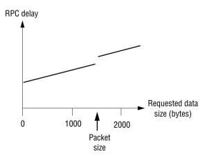
Figure 7.12 shows, schematically, client delay against requested data size. The delay is roughly proportional to the size until the size reaches a threshold at about network packet size. Beyond that threshold, at least one extra packet has to be sent, to carry the extra data. Depending on the protocol, a further packet might be used to acknowledge this extra packet. Jumps in the graph occur each time the number of packets increases.
