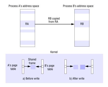
Copy-on-write is a general technique – for example, it is also used in copying large messages – so we take some time to explain its operation here. Let us follow through an example of regions RA and RB, whose memory is shared copy-on-write between two processes, A and B (Figure 7.4). For the sake of definiteness, let us assume that process A set region AB to be copy-inherited by its child, process B, and that the region AB was thus created in process B.
