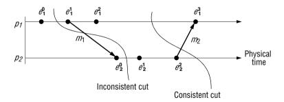
Each event either is an internal action of the process (for example, the updating of one of its variables), or is the sending or receipt of a message over the communication channels that connect the processes.
