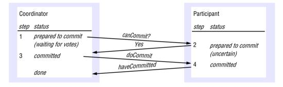
used by its transaction cannot be released for use by other transactions. The participant can make a *getDecision* request to the coordinator to determine the outcome of the transaction. When it gets the reply, it continues the protocol at step 4 in Figure 17.5. If the coordinator has failed, the participant will not be able to get the decision until the coordinator is replaced, which can result in extensive delays for participants in the *uncertain* state.
