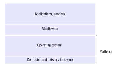
interactions with each other. Given the complexity of distributed systems, it is often helpful to organize such services into layers. We present a common view of a layered architecture in Figure 2.7 and develop this view in increasing detail in Chapters 3 to 6.
