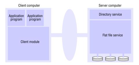
distributed system. When the flat file service receives a request to create a file, it generates a new UFID for it and returns the UFID to the requester.
