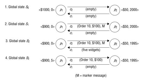
processes have the initial states shown in Figure 14.11. Process  $p_2$  has already received an order for five widgets, which it will shortly dispatch to  $p_1$ .
