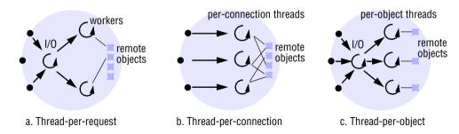
objects. The *thread-per-object architecture* (Figure 7.6c) associates a thread with each remote object. An I/O thread receives requests and queues them for the workers, but this time there is a per-object queue.
