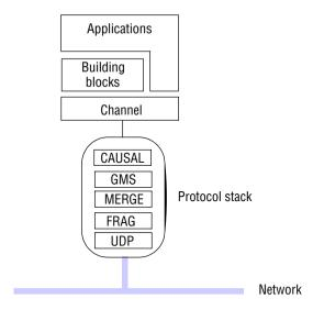
• The *protocol stack* provides the underlying communication protocol, constructed as a stack of composable protocol layers.
