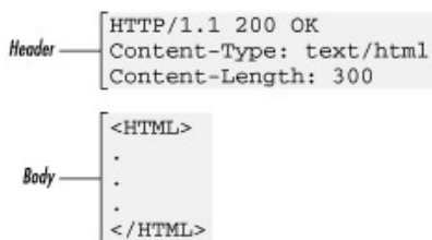
Figure 2-3. The HTTP header/body message structure
