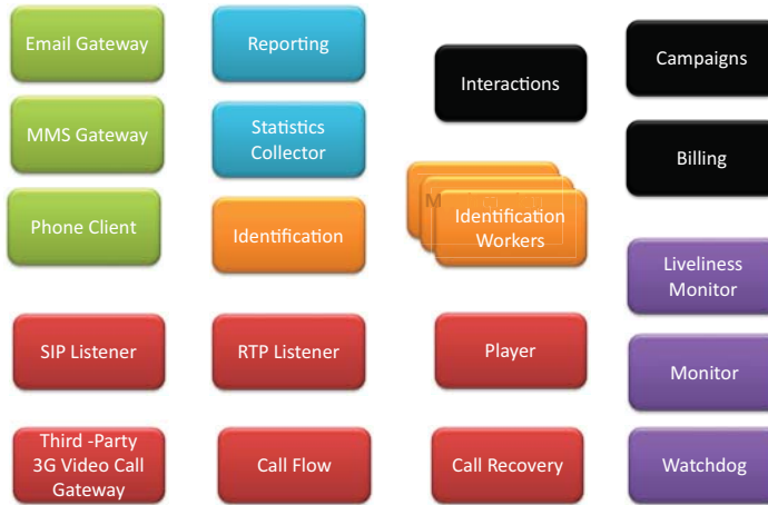
Figure 9.2 Some of the services in the system that implement business services. Providing identification by email involves several services: the Email Gateway, Identification (with its ID Workers), Watchdog, Statistics Collector, Monitor, and Billing. The discussion of the solution will use these services in different contexts to demonstrate different patterns.
