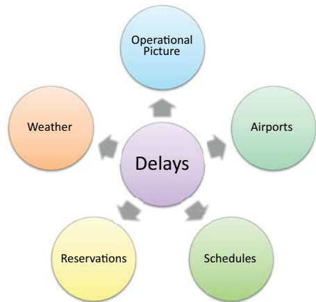
Figure 5.9 Some of the services that a Delays service would need to interact with. The Delays service drives some of the services directly (such as Reservations and Schedules) but it's driven by data coming from the other services (Weather, Operational Picture, and Airports).
