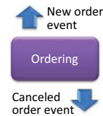
Figure 8.4 The Ordering service using the Inversion of Communications pattern. Now the service doesn't know about or depend on other services directly. It's only aware of two business events—new order and canceled order—which are relevant to the business function that the service handles.
