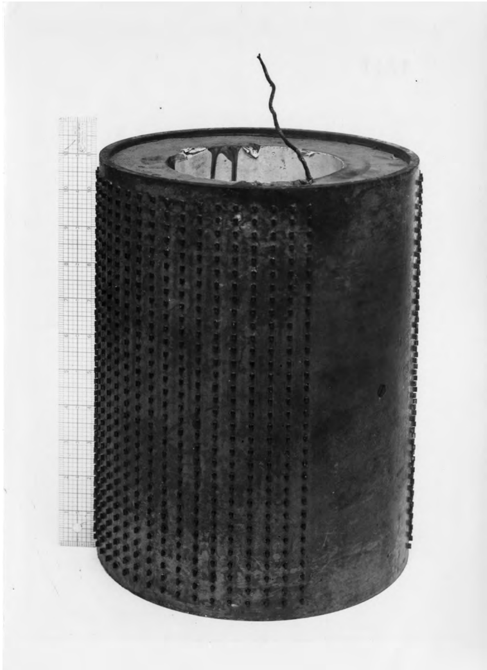
Figure 1.15 The Atanasoff-Berry Computer's memory drum—the sole surviving component. (Source: Iowa State Univ. Library Special Collections and Univ. Archives.)
