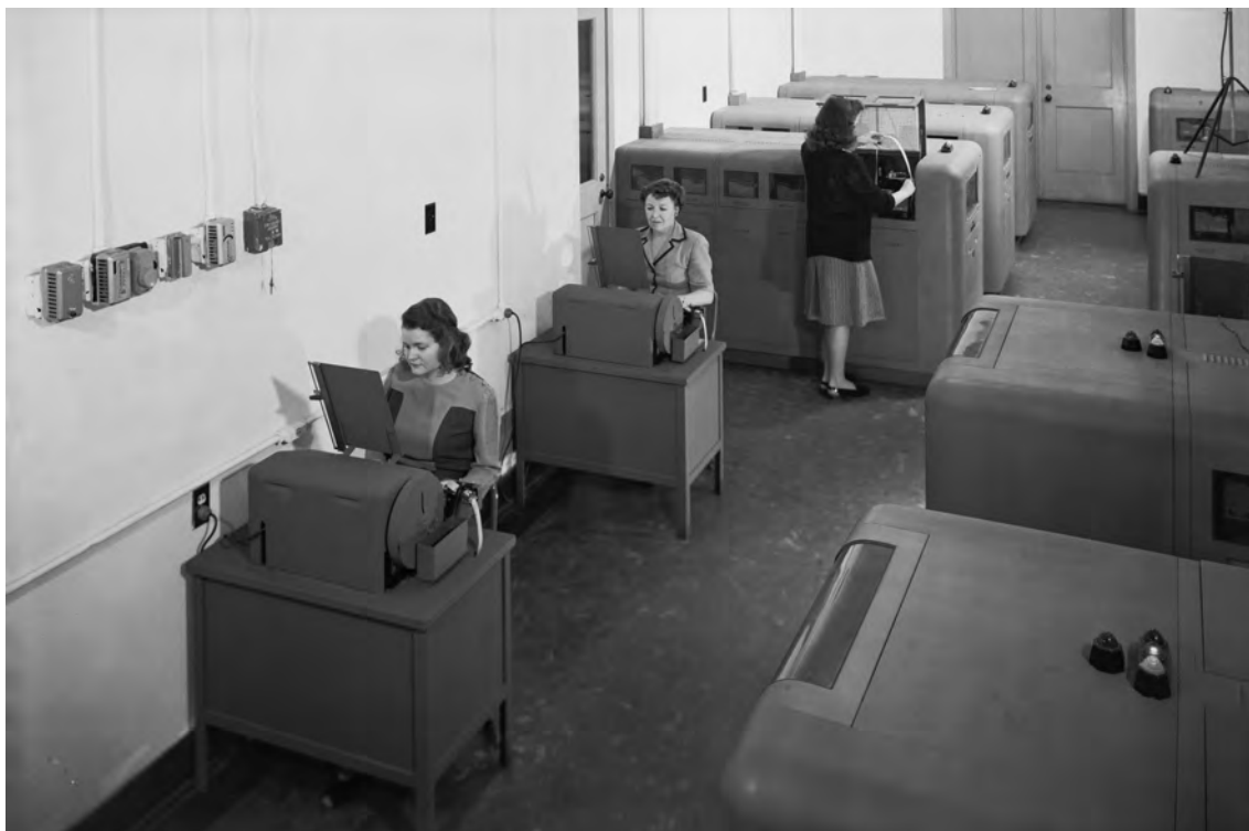
Figure 1.8 Bell Labs relay computers in use at Langley Research Center (1947) by female “computers” who performed mathematical computations for male staff. Note: the actual relay computer is not shown (these are the input/output devices). (Source: NASA, credit: NACA Langley.)
