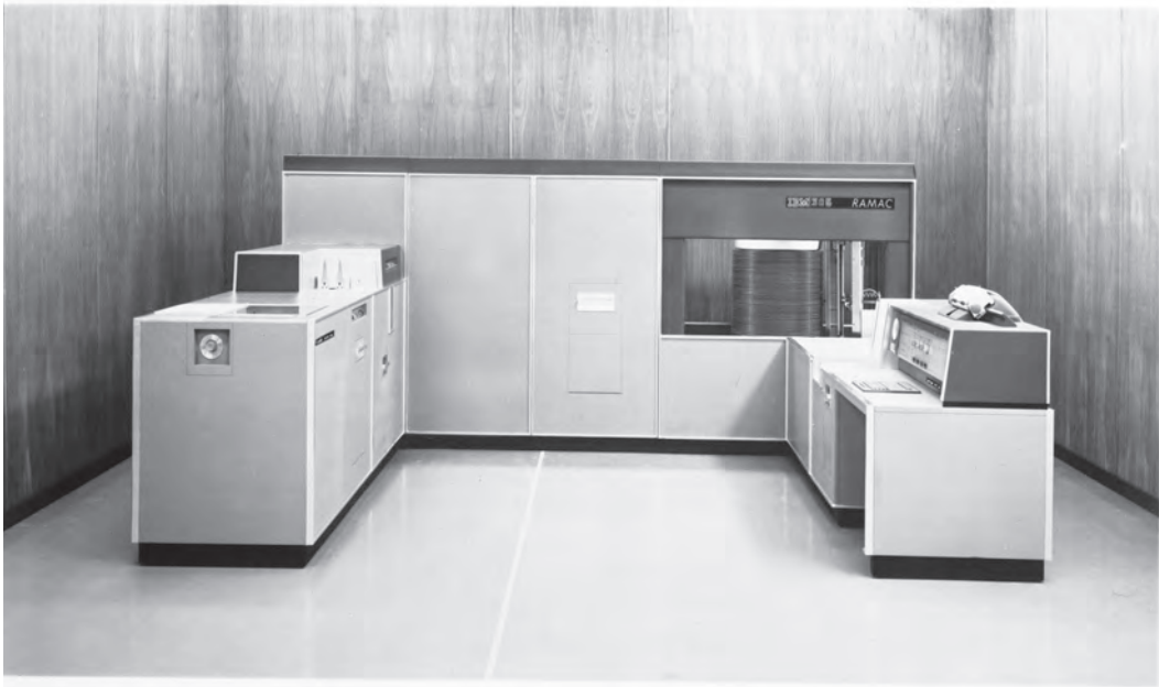
Figure 7.1 The IBM 350 disk storage unit stored 5 million 6-bit characters in 1956. Note the actual disk platters are in the back right and were visible through the window. (Source: Courtesy of International Business Machines Corporation, ©International Business Machines Corporation.)
