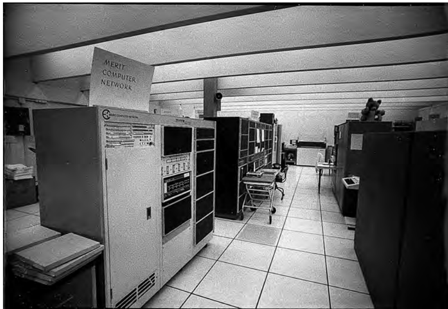
Figure 6.8 A front-end processor (MM-16) to communicate to a DEC PDP-11 for the MERIT network at University of Michigan in 1982. (Source: Courtesy of MERIT Network.)
