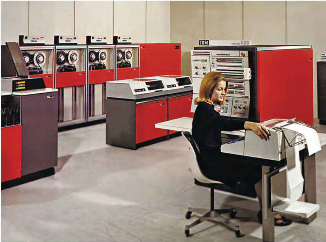
Figure 3.4 IBM System/360 model 40 with woman at console and assorted disk drives, tape drives, and card reader, circa 1964. (Source: Courtesy of International Business Machines Corporation, ©International Business Machines Corporation.)
