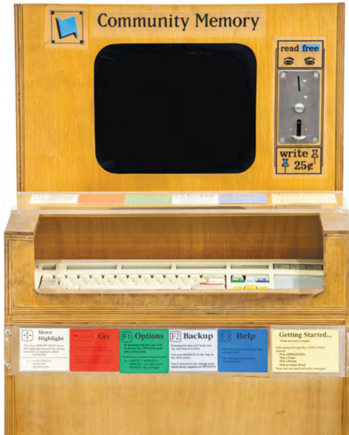
Figure 6.10 Community memory, public terminal for BBS in Berkeley, CA, 1975. (Source: Mark Richards. Courtesy of the Computer History Museum.)
