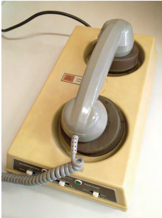
Figure 6.5 An AM211 CXR Anderson Jacobson acoustic modem (French version) and the phone handle (almost) plugged in. (Source: Olivier Berger, CC BY-SA 3.0 https://creativecommons.org/licenses/by-sa/3.0 , via Wikimedia Commons and with permission of CXR Anderson Jacobson.)
