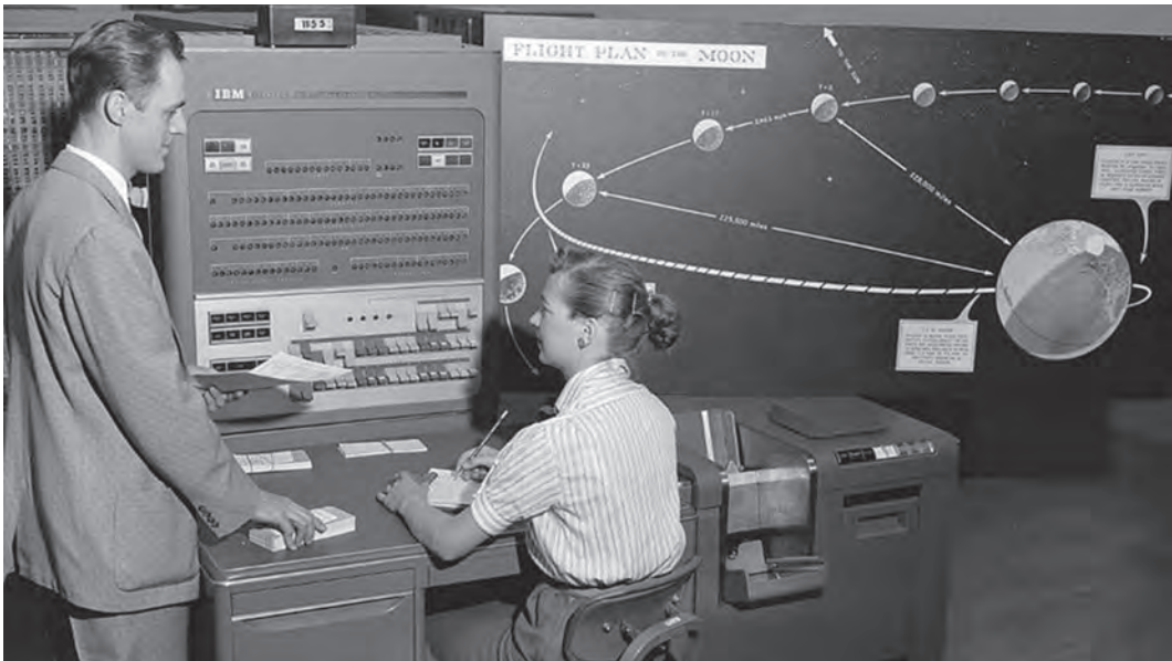
Figure 3.1 IBM 704 at NASA's Jet Propulsion Laboratory in 1959 with an unknown human “computer” seated at the console with a card reader/punch to the right. (Source: Courtesy of International Business Machines Corporation, ©International Business Machines Corporation.)
