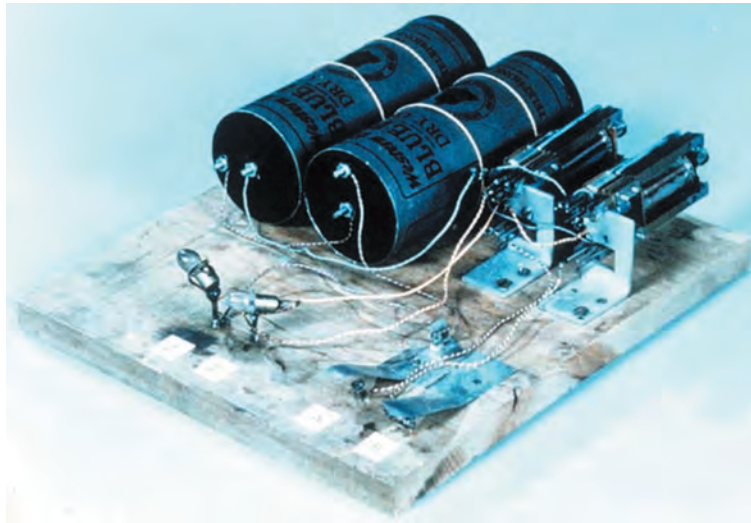
Figure 1.9 Stibitz reconstruction of Bell Labs “Kitchen” Model, original built in 1936. (Source: Courtesy of AT&T Archives and History Center.)
