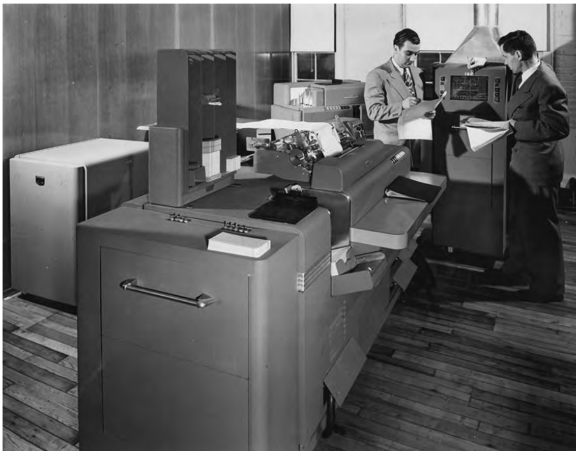
Figure 1.17 The IBM Card-Programmed Electronic Calculator was the first digital computer used by the US space program. (Source: Courtesy of International Business Machines Corporation, ©International Business Machines Corporation.)
