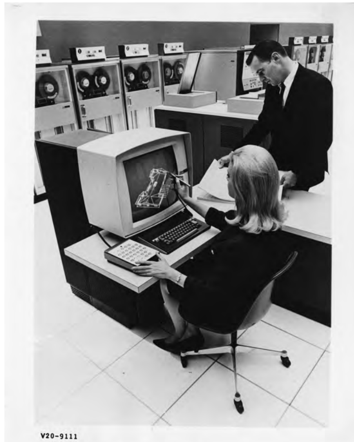
Figure 8.5 IBM System 360 Model 40 demonstrating a drawing system using a lightpen. (Source: Courtesy of International Business Machines Corporation, ©International Business Machines Corporation.)
