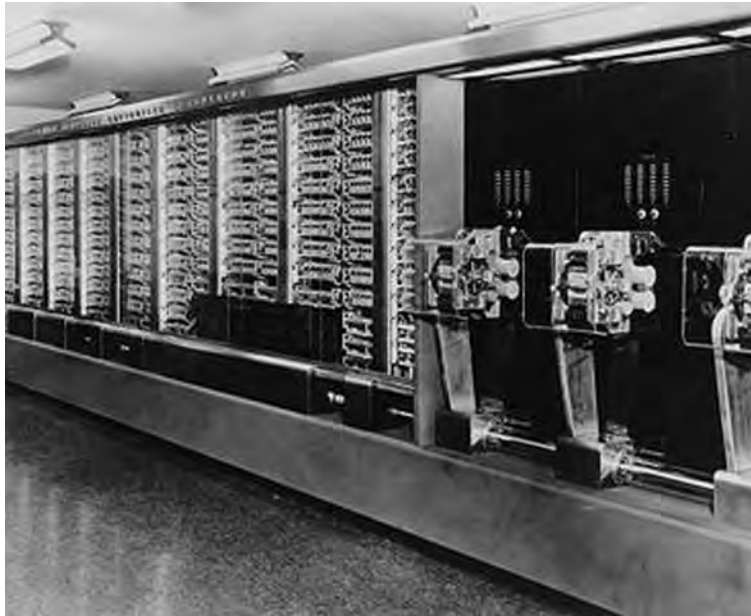
Figure 1.14 IBM ASCC (or Harvard Mark I, undated). (Source: Courtesy of International Business Machines Corporation, ©International Business Machines Corporation.)
